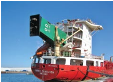
The vessel's damaged superstructure after the collision with the bridge
