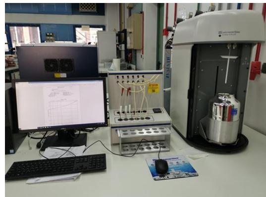
High-performance adsorption analyzer for measuring surface area, pore size, and pore volume of powders and particulate materials.
