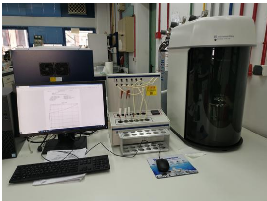
High-performance adsorption analyzer for measuring surface area, pore size, and pore volume of powders and particulate materials.
