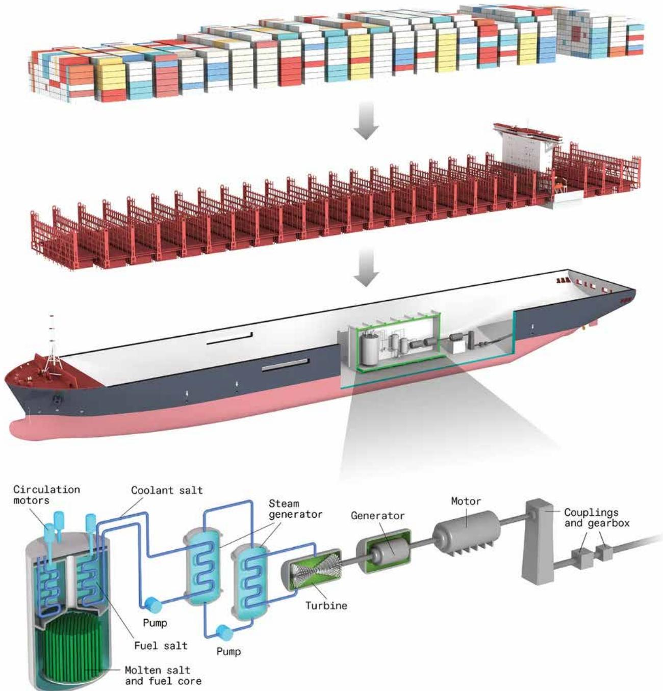
Image 6a: Artistic renderings of a nuclear container ship featuring molten salt reactors (Molten Salt Reactor - MSR) <sup>31</sup>
