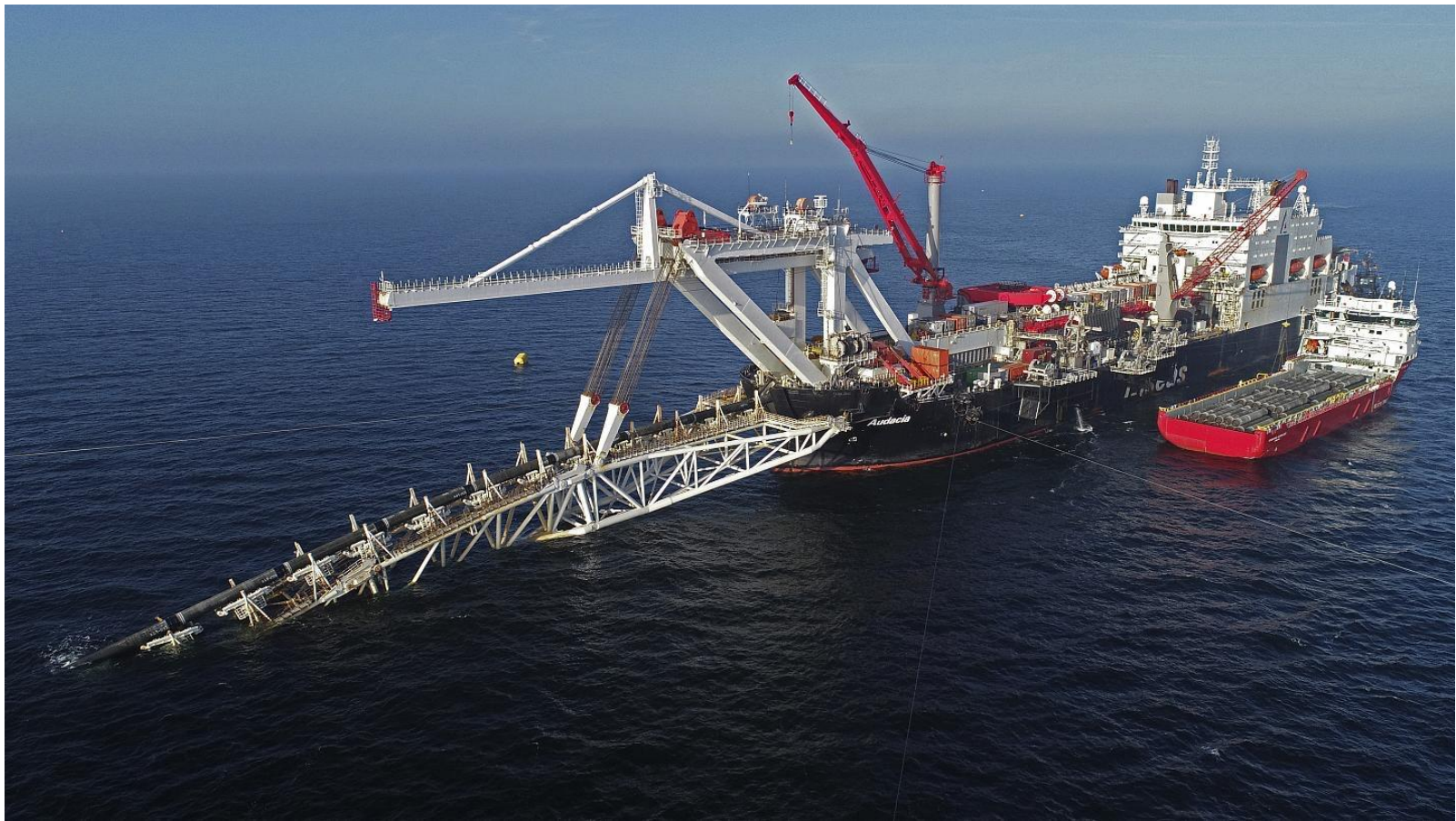
A specialized barge lays pipe under the Baltic Sea in 2019 for the controversial Nord Stream 2 pipeline, which is meant to carry additional Russian gas to Germany
