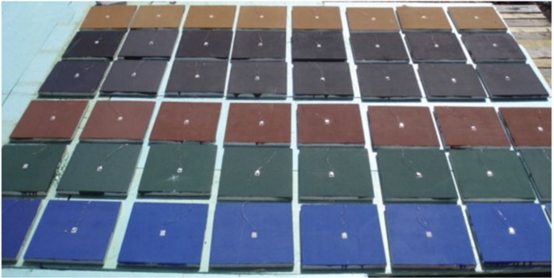
Tested tiles coated with common, cool and PCM coatings
