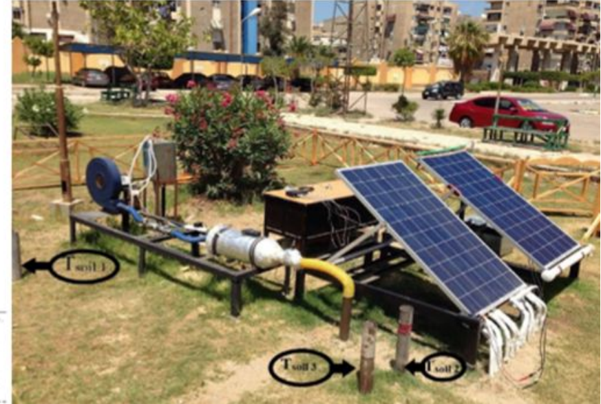
Schematic diagram and experimental setup of hybrid EAHE coupled with PVT collector
