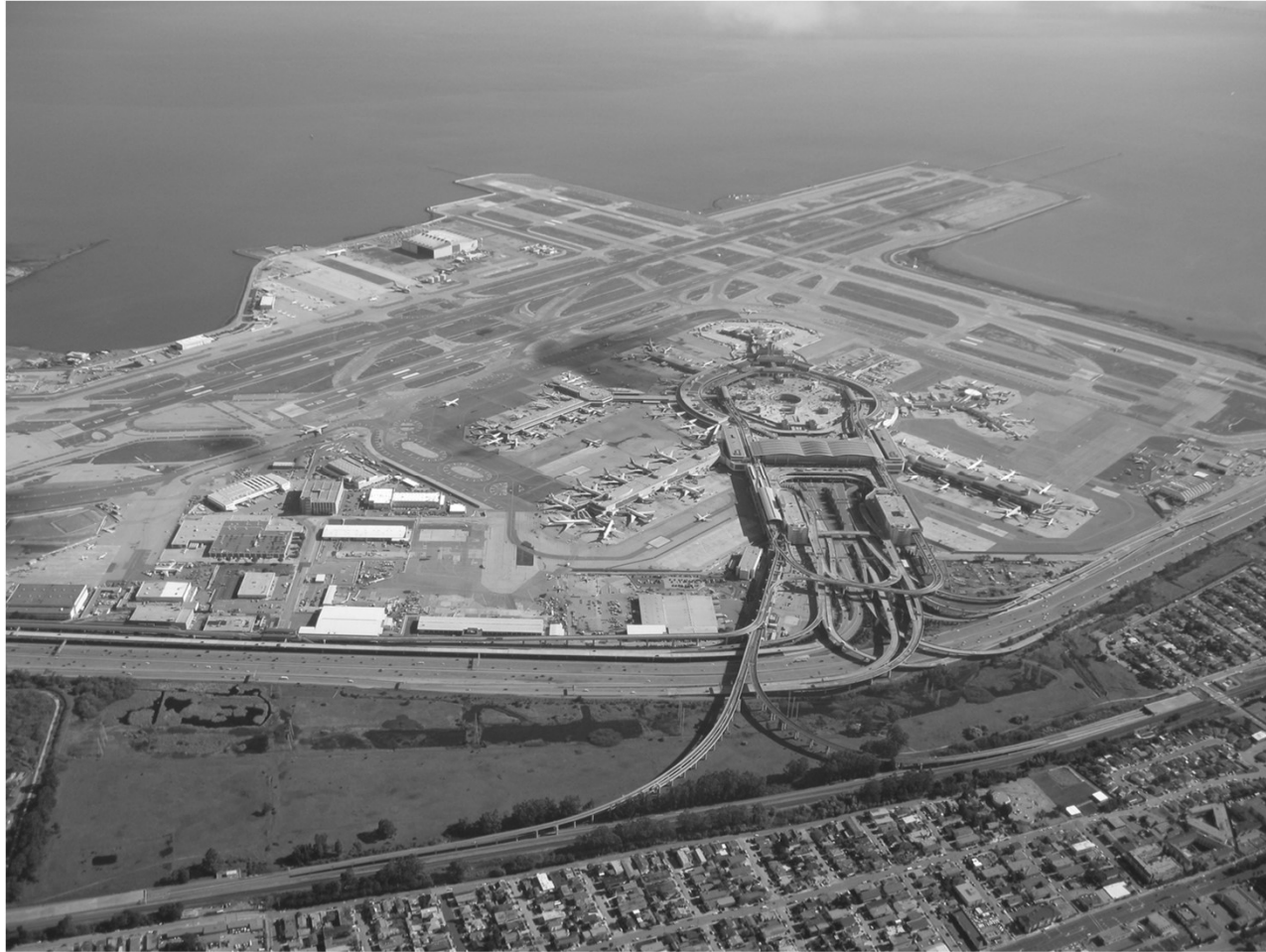
The San Francisco Airport (U.S.) has intersecting runways that interfere with one another. Source: unknown
