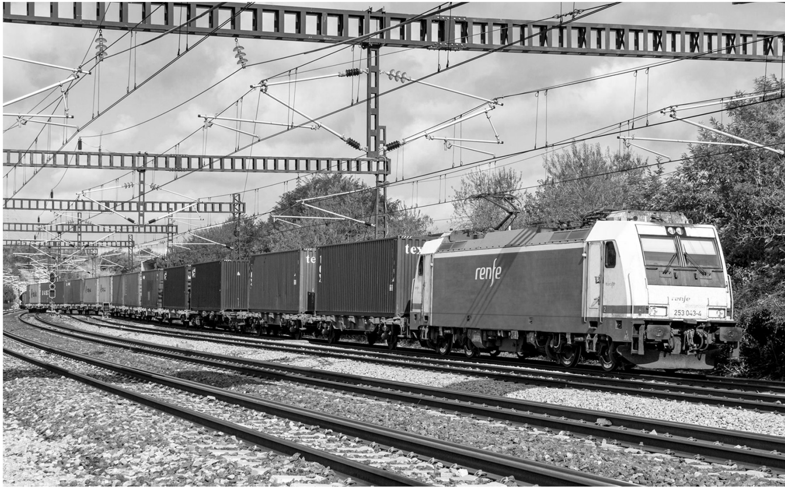
A single-stack train in Spain, limited in height by the electric catenaries.
