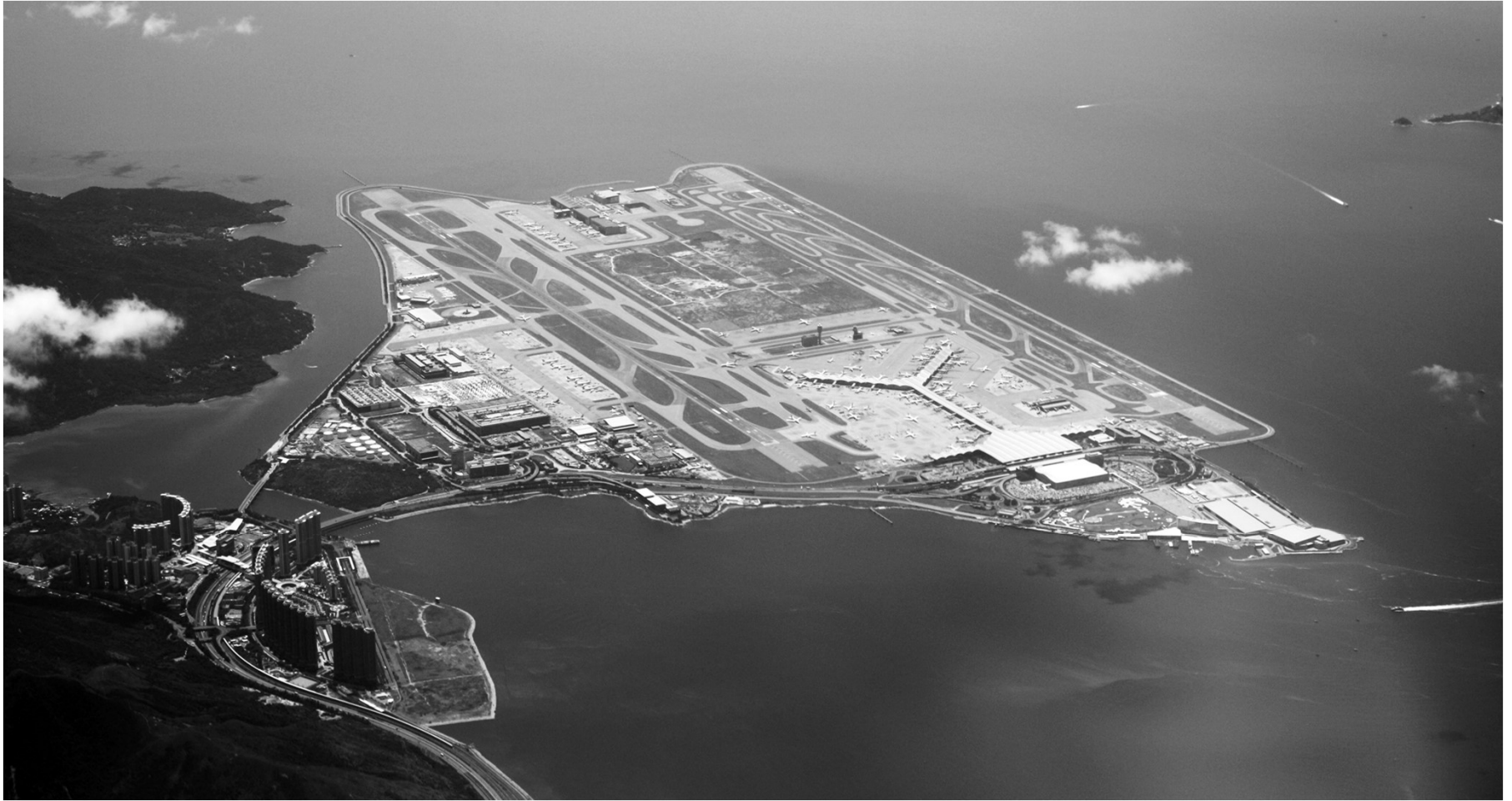
The new Chek Lap Kok Airport (Hong Kong) was built on an artificial island. Source: Wylkie Chan
