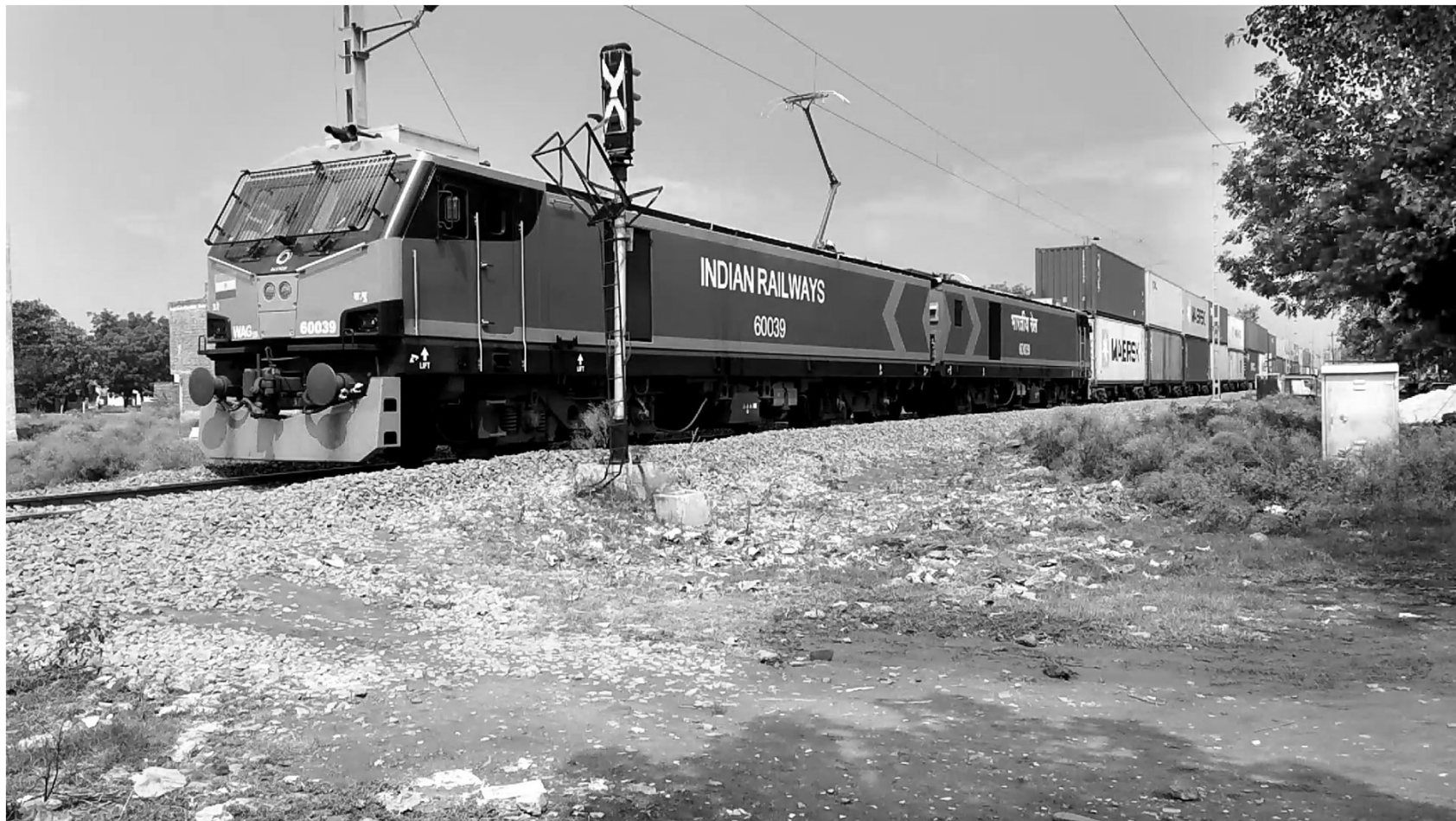
A double-stack train under electric catenaries on a high-speed rail line in India. Source: Indian Railways
