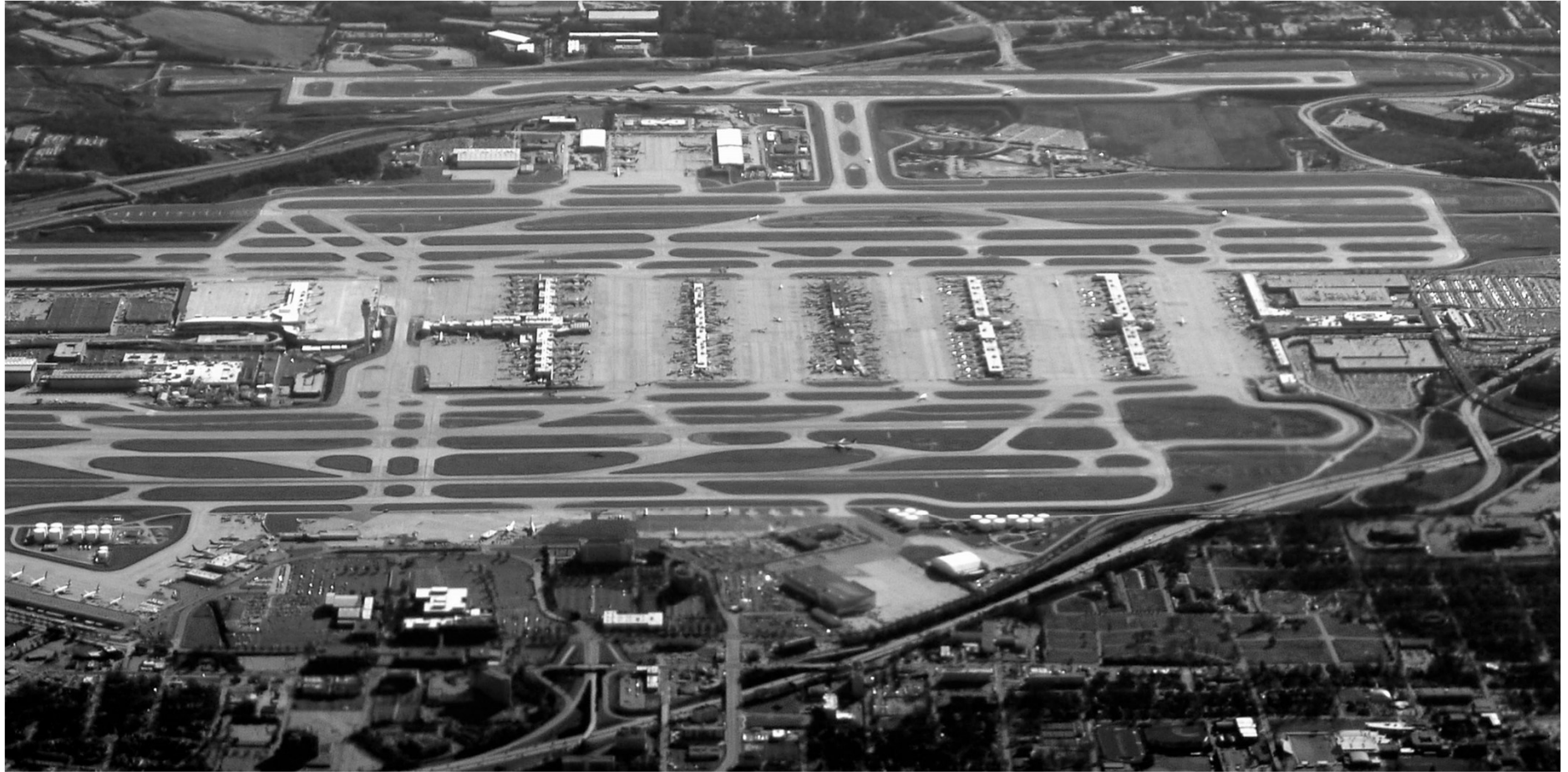
The Atlanta Airport (U.S.) has parallel runways that do not interfere with one another. Source: unknown
