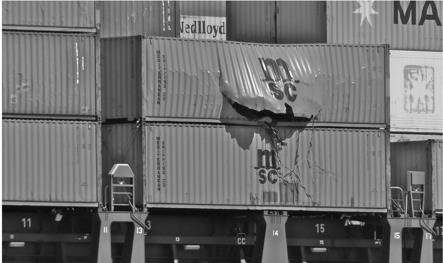
Cargo that is poorly secured in a container can be lost at sea. Source: Will Van Dorp
