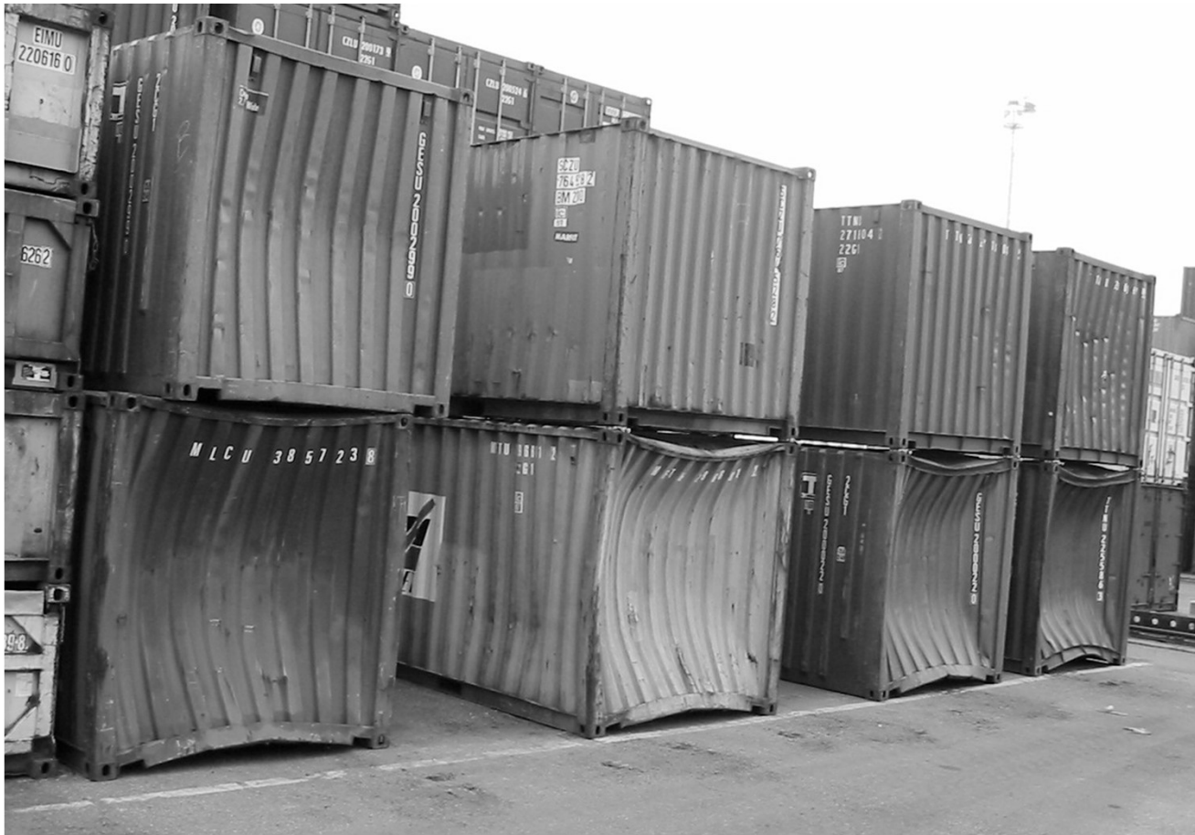
Waves can damage containers, even though they are made of very strong steel. Source: Danny Cornelissen
