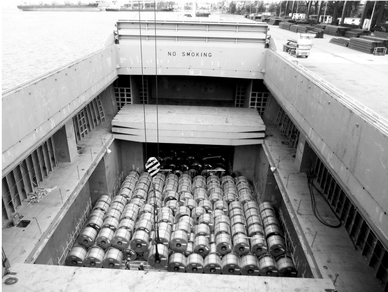
A general-cargo ship carries breakbulk cargo that is placed directly in the holds of the ship. Source: Wathit Kettap
