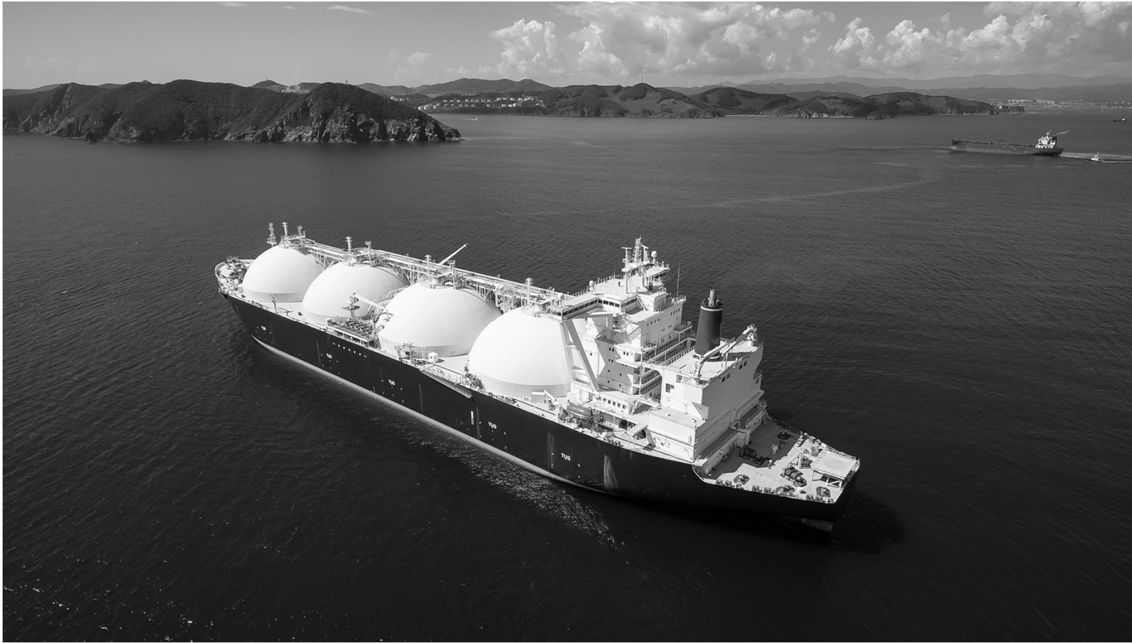
A liquefied natural gas carrier with its characteristic spherical tanks. Source: Vladimir Serebryanskiy
