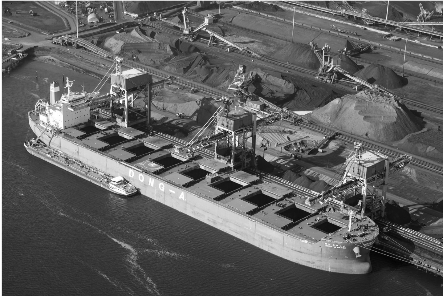
A dry-bulk carrier with hatches open, loading coal in Australia. Source: Aerovista Luftfotographie
