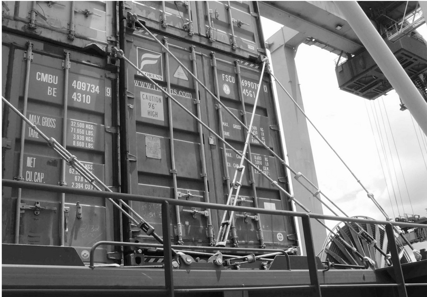
Containers placed on the deck of containerships are tied to the ship by lash bars and twist locks. Source: Ole Tange
