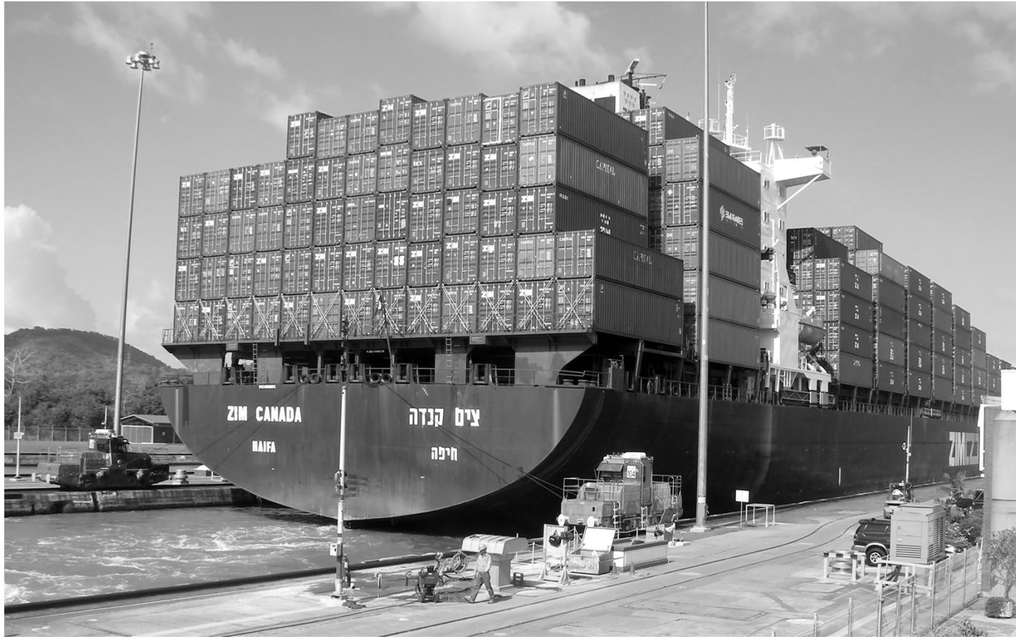
A Panamax containership in the Panama Canal locks, easily identifiable by its 13 containers abreast.
