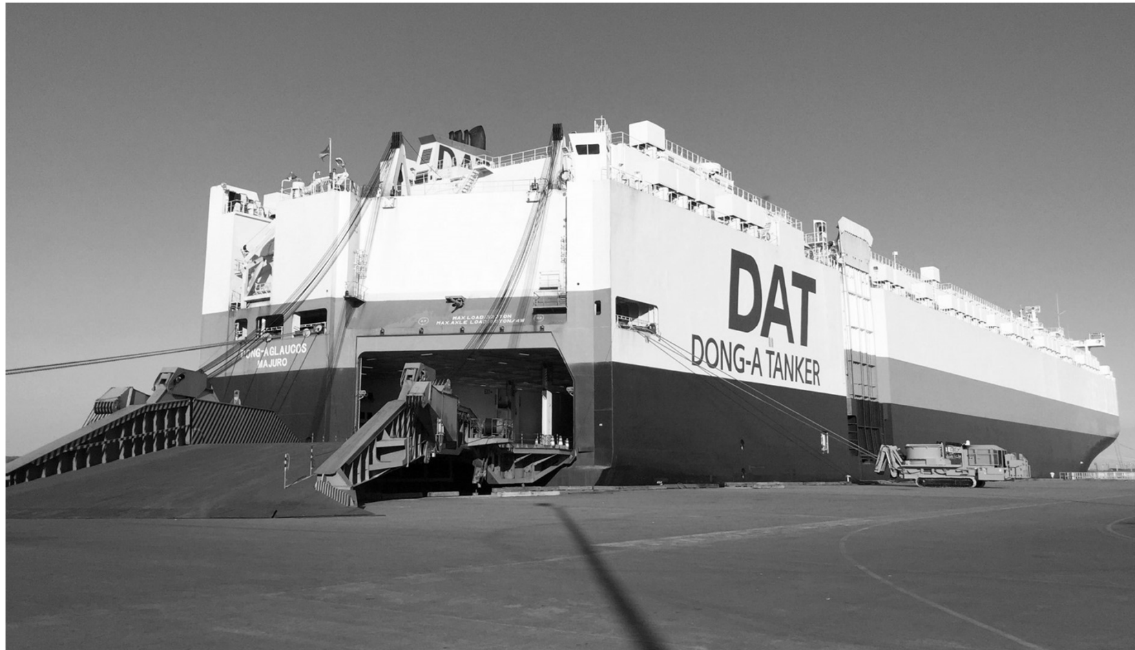
A roll-on roll-off [RORO] ship allows wheeled cargo to be driven onboard the ship with a ramp. Source: James R. Martin
