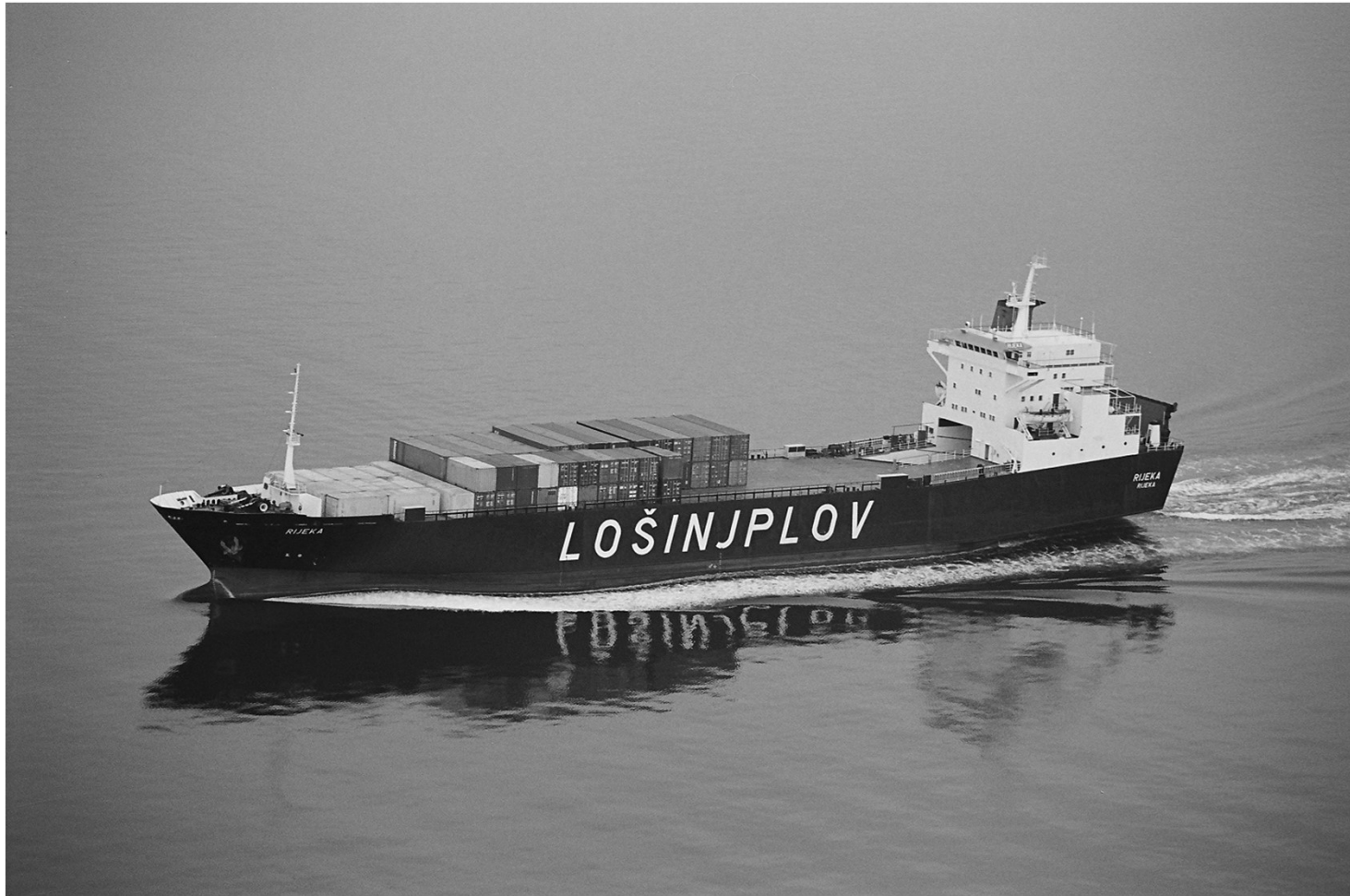
A combination ship carries containers, breakbulk, and roll-on roll-off cargo. Source: Losinjska Plovida
