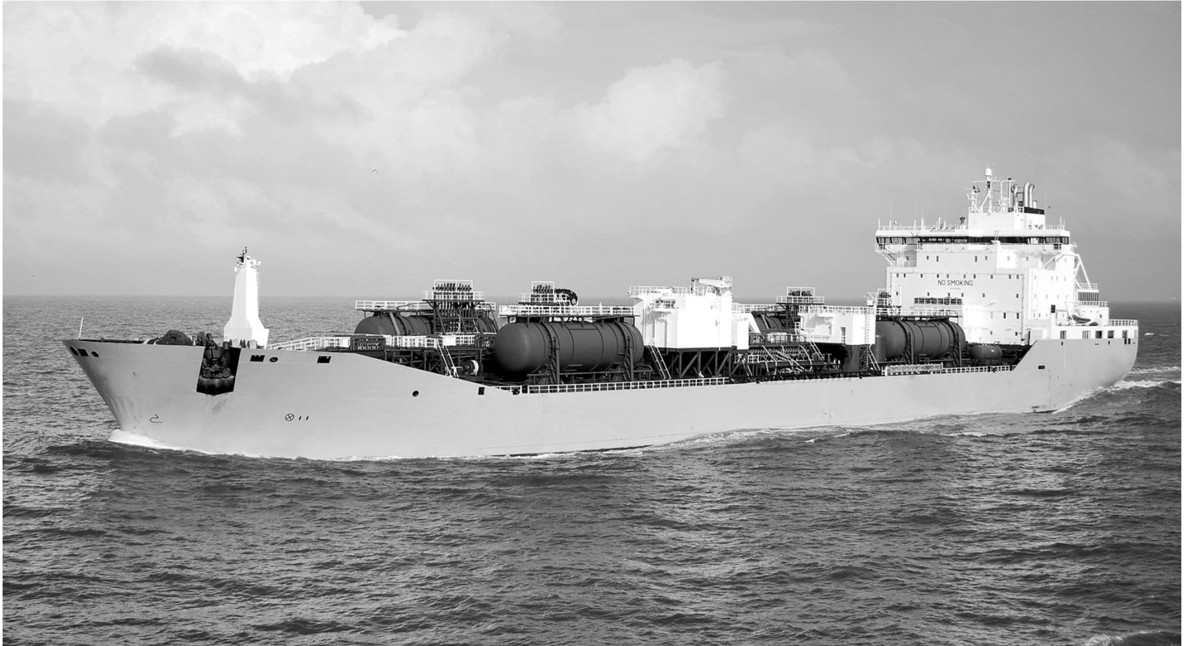
A product carrier (chemical carrier) with its network of pipes and tanks. Source: Andrejs Polivanovs
