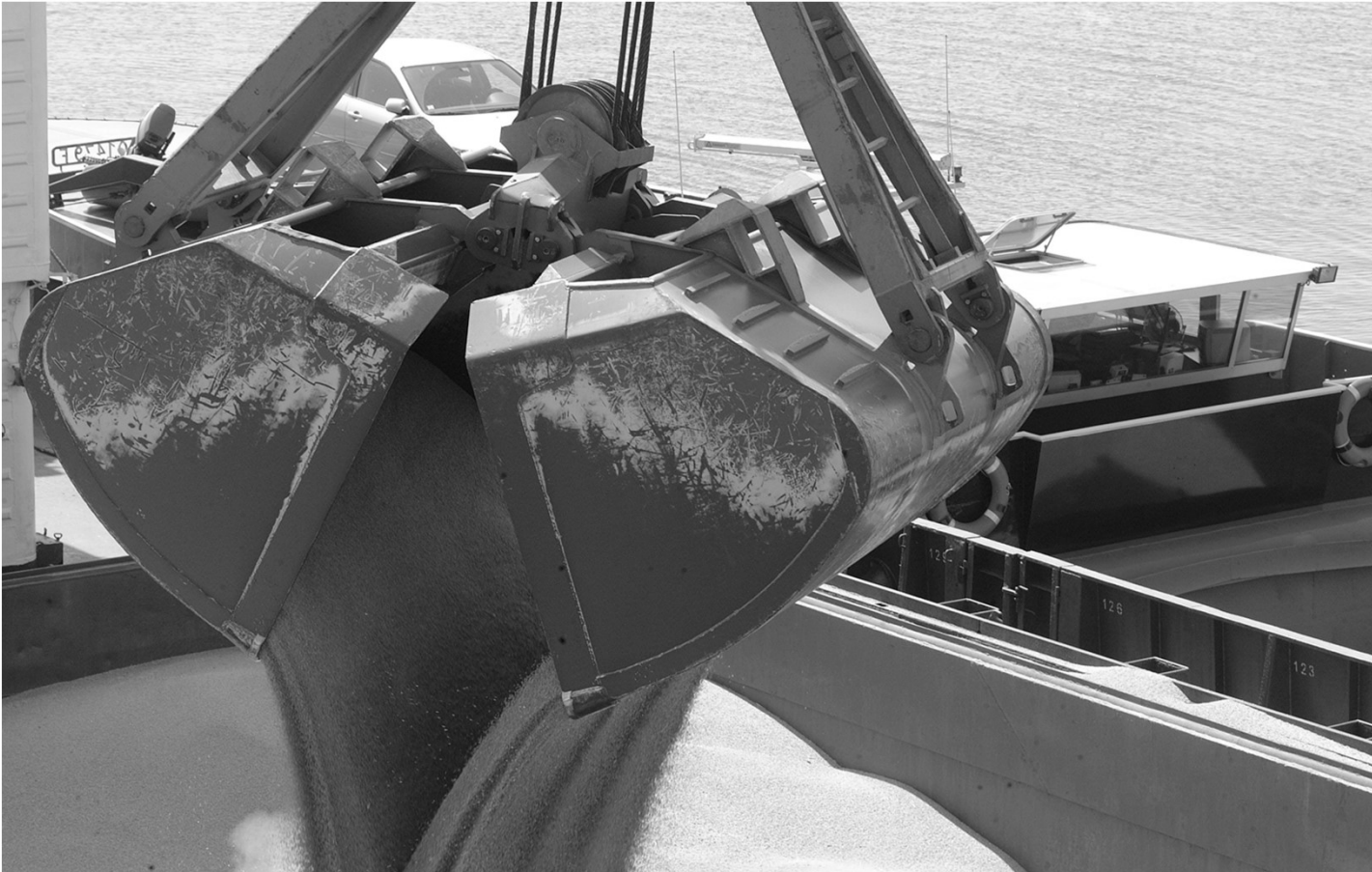
Dry-bulk cargo is placed directly into the holds of a ship and fills them like a liquid would. Source: unknown
