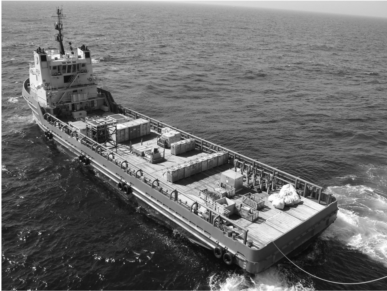
A supply ship, used to provide support to oil platforms and other ships at sea. Source: unknown
