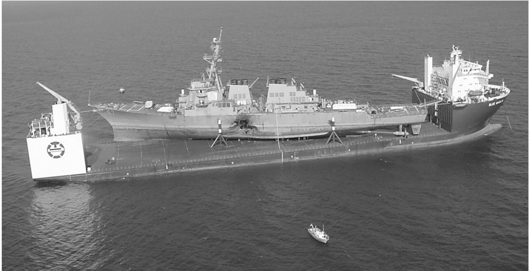
A heavy-lift ship, used to transport very large cargo. The MV Blue Marlin . Source: unknown
