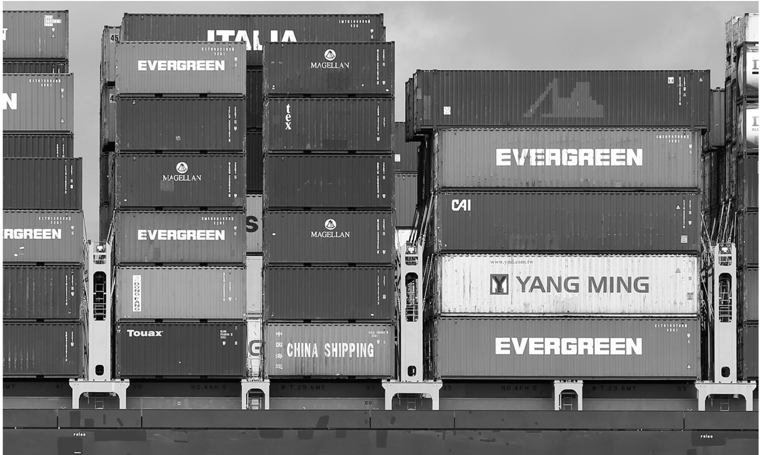
Containers aboard a containership. 20-footers on the left, 40-footers on the right, with a 45-foot container on the top of the stack on the right.
