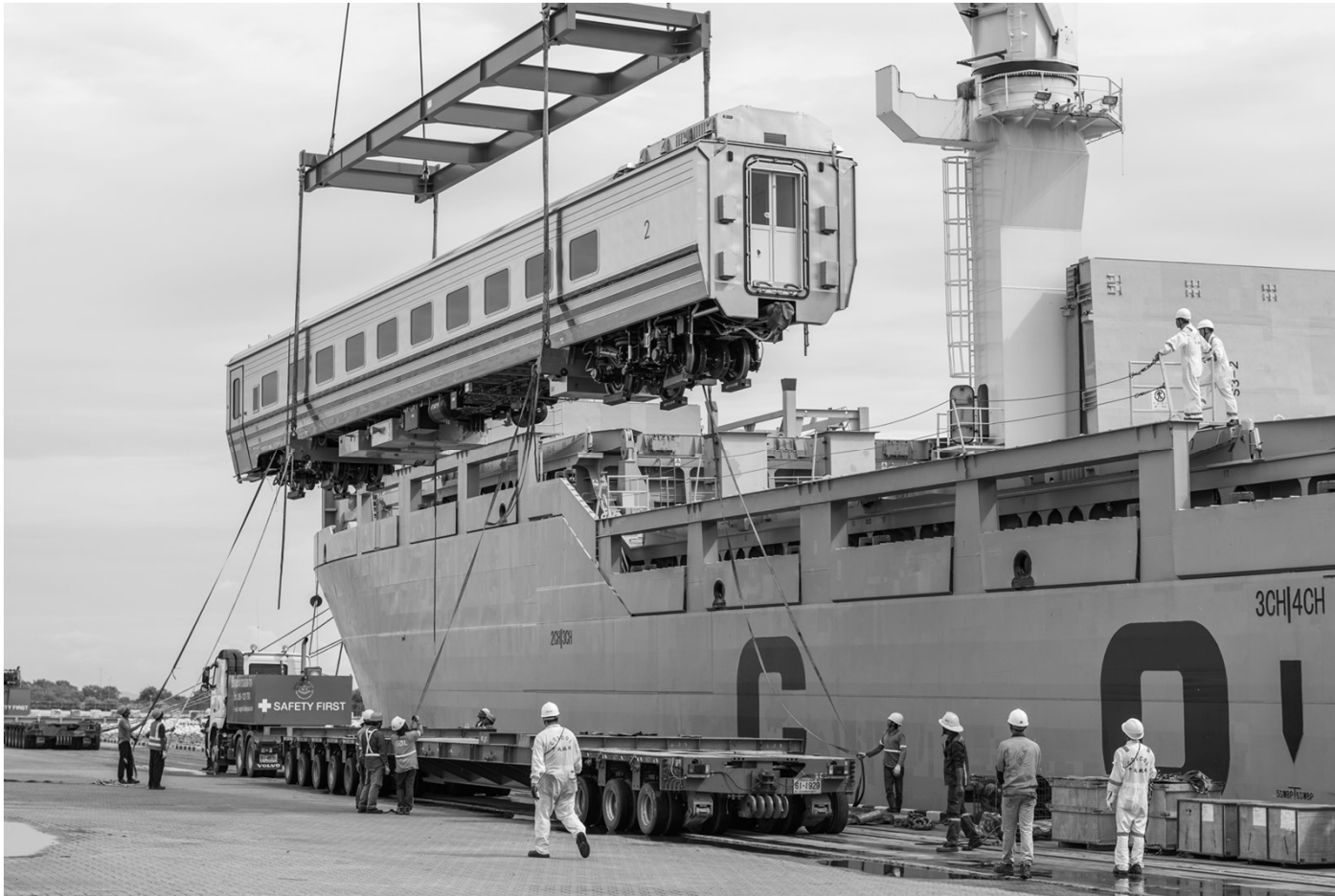
Breakbulk cargo is either too heavy or too large to be placed in a container. Source: May Chanikran
