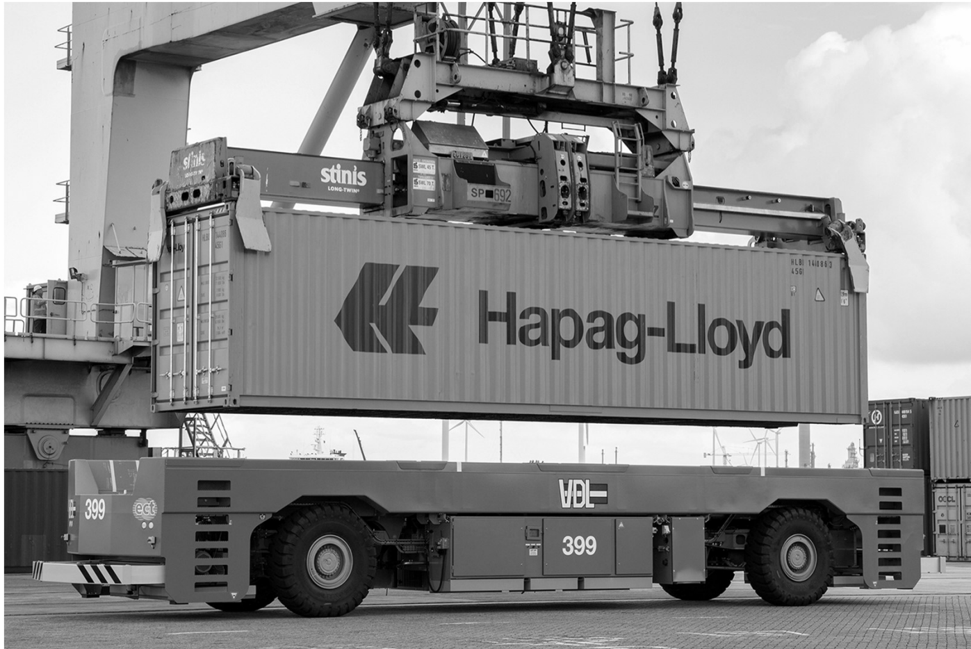
Automated Guided Vehicles (AGVs) transport containers between the yard and the quay cranes in the Port of Amsterdam.
