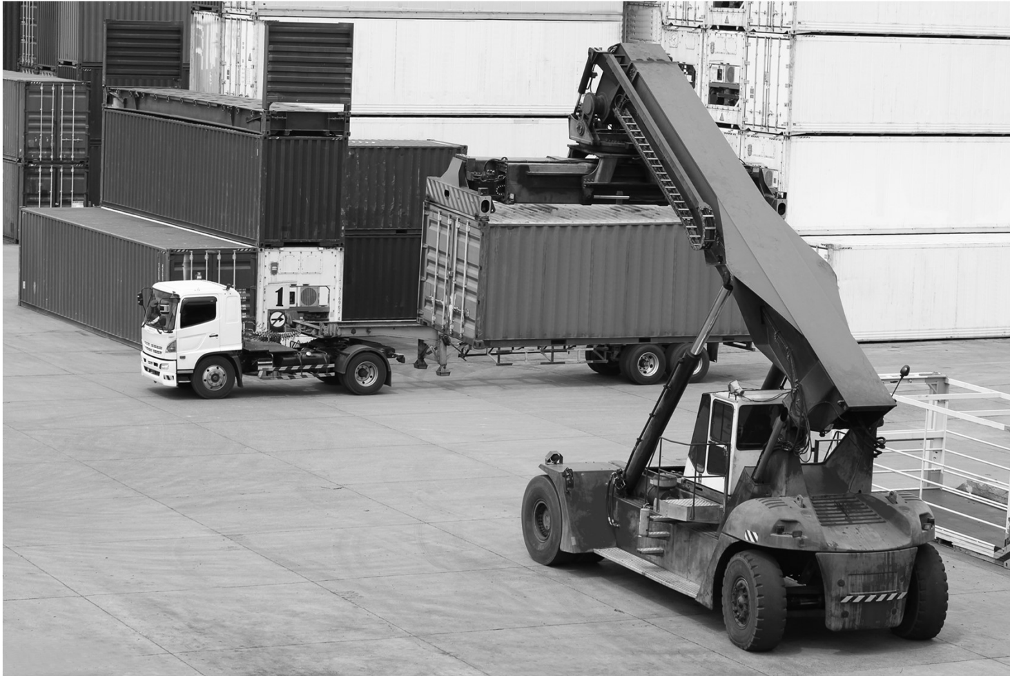
Container stackers move containers from trucks to the container yard. Source: Sanit Fuangnakhon
