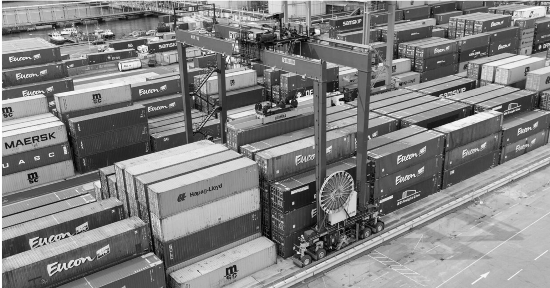
Rubber-tired gantry cranes move containers in the container yard.
