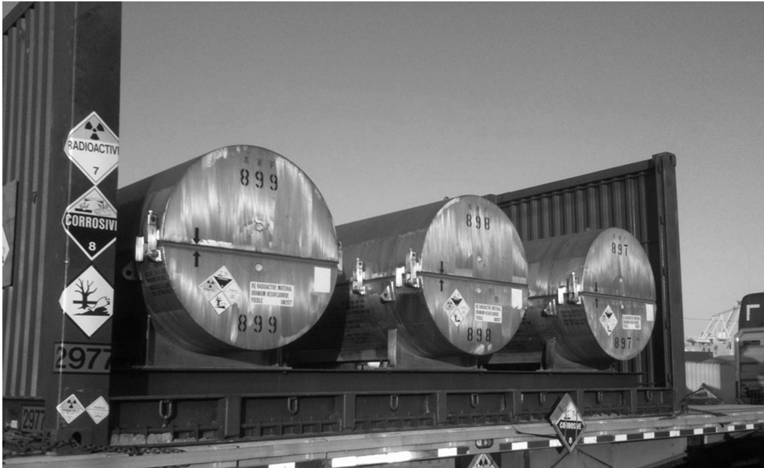
A shipment of radioactive and corrosive material that is dangerous to wildlife (uranium hexafluoride)
