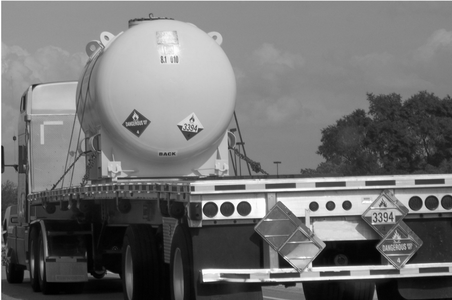
A truck transporting flammable solids that are both pyrophoric and flammable when wet. Source: Daniels Training Services
