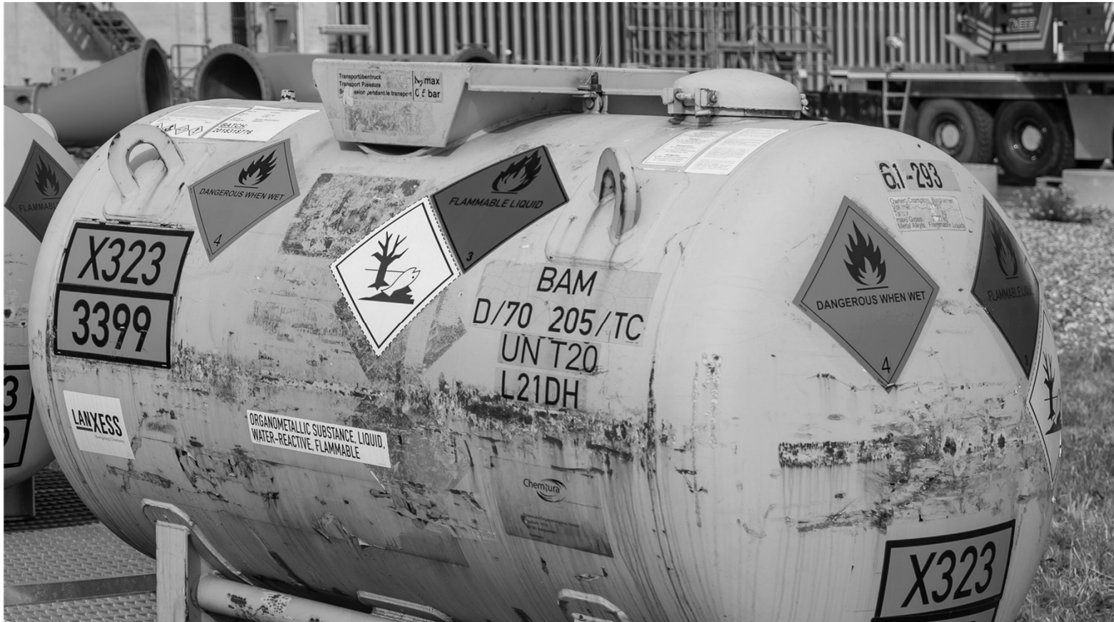
A container of a flammable liquid that is also flammable when wet. Source: Uwe Aranas
