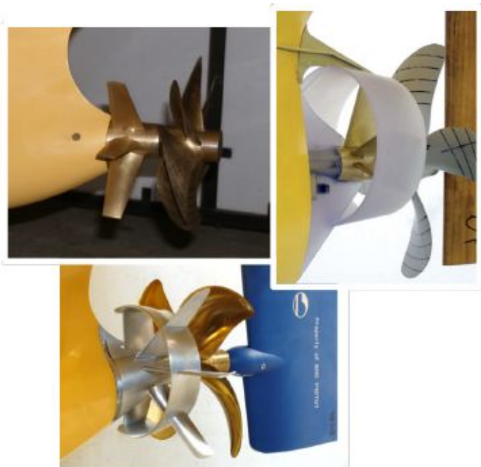
Pre-Swirl Devices: top left, Pre-Swirl Stator (PSS); top right, Pre-Swirl Duct (PSD, e.g. Becker Mewis Duct), bottom; Becker Mewis Duct Twisted (BMDT, specifically suited for container vessels)
