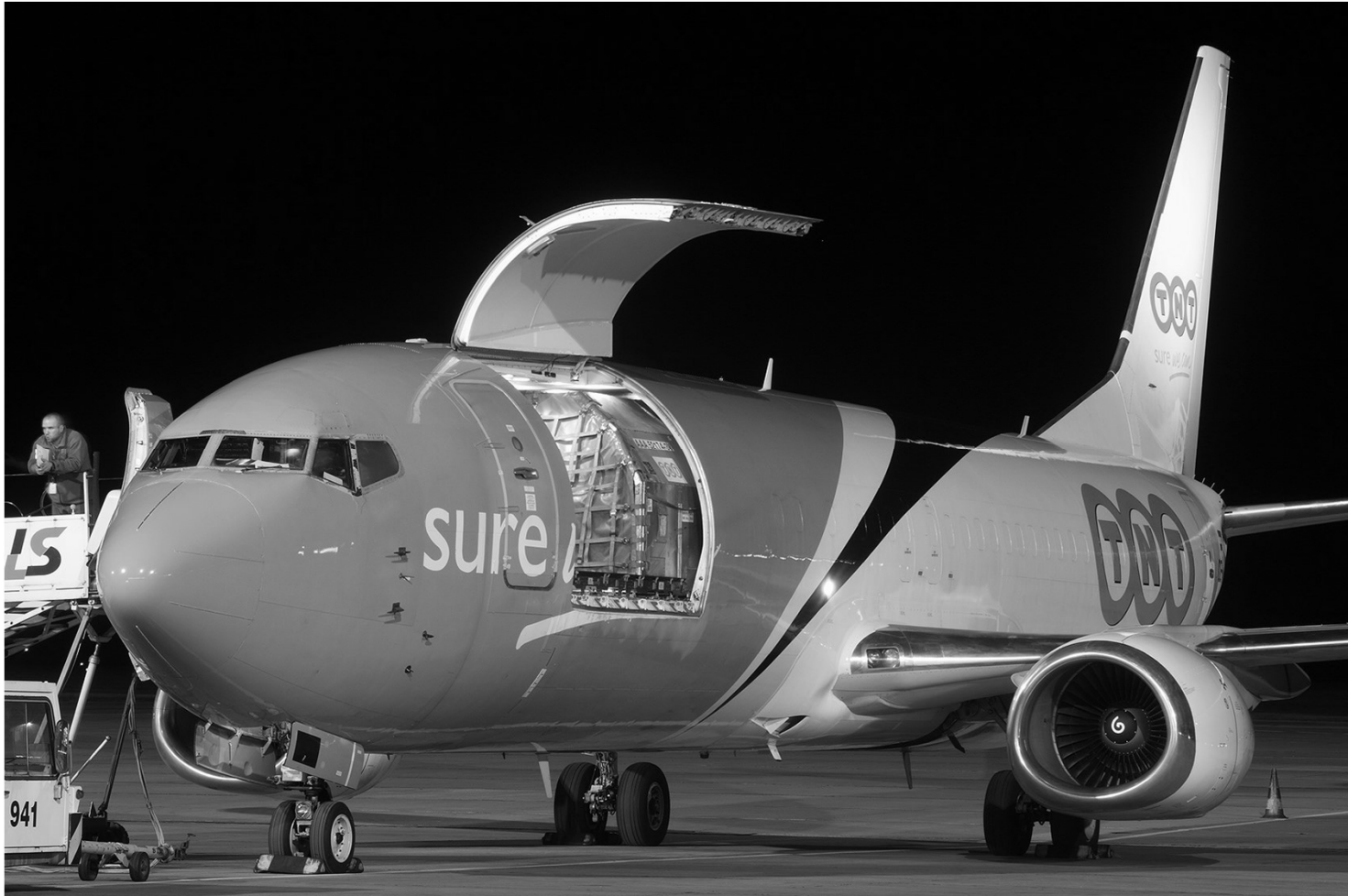
Cargo can be loaded through a side door (Boeing 737, converted from passenger to cargo). Source: unknown
