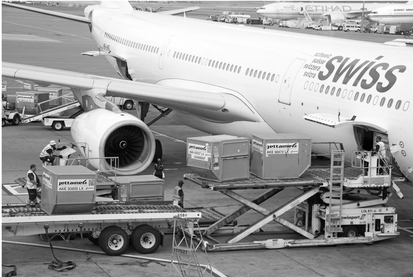
Cargo being loaded in the belly of an Airbus A 330 passenger aircraft. Source: Peter Titmuss
