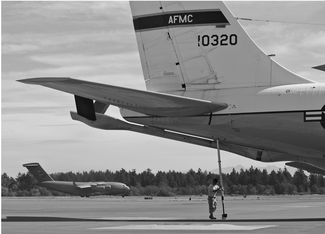
Airfreighters can be loaded more easily if their tail is stabilized, so that they do not tip over. Source: US Air Force
