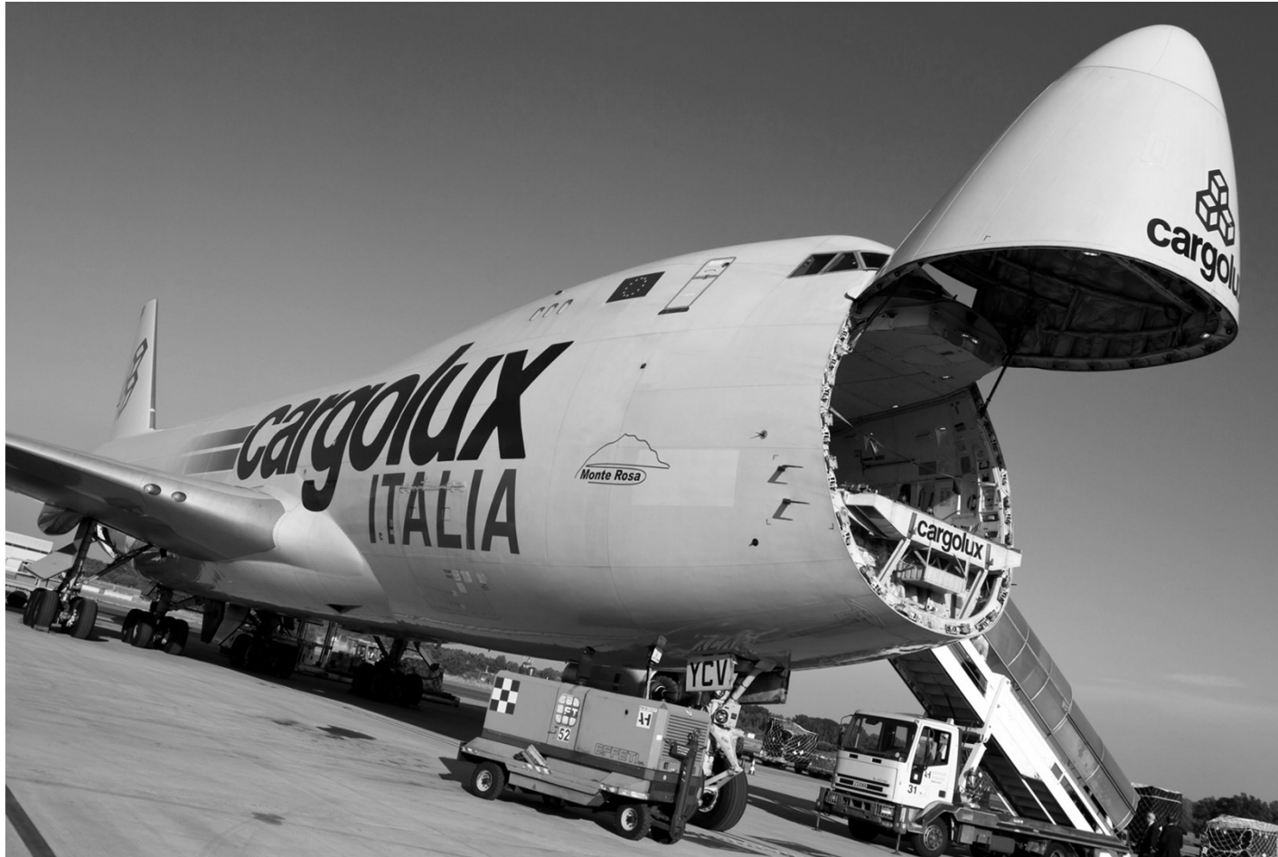
An airfreighter can be loaded through its nose (Boeing 747F). Source: Tratong
