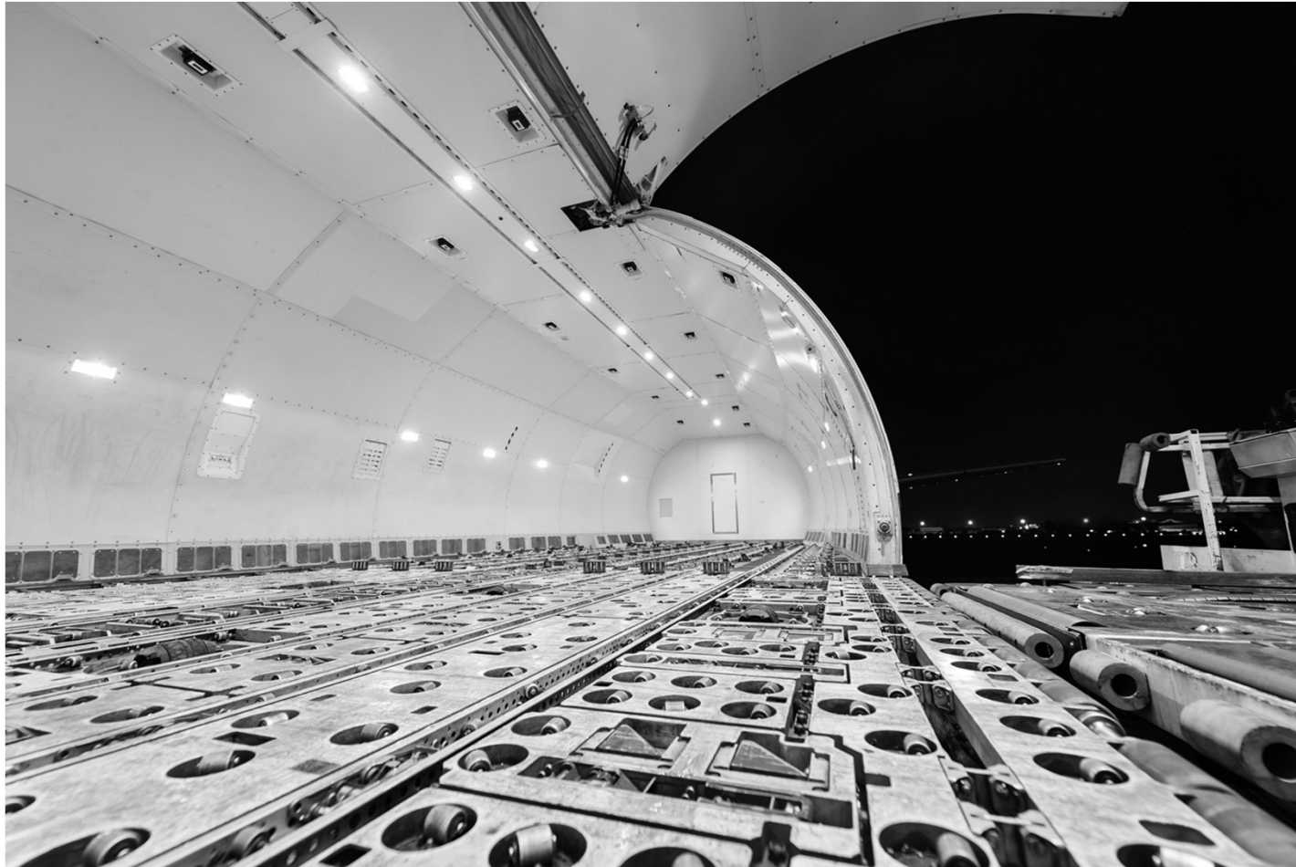
An airfreighter carries cargo on its main deck. The roller deck of an Airbus 330F. Source: Tratong
