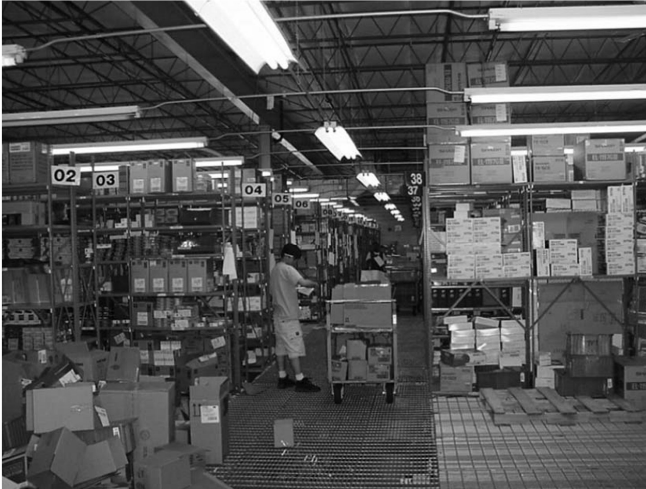
A picker retrieving multiple orders using a paper list in a cluster-picking warehouse (several orders picked at once).
