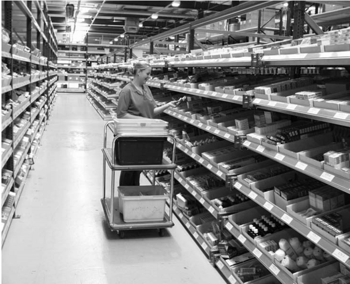
A picker-to-goods strategy asks the picker to move through the warehouse. Source: unknown
