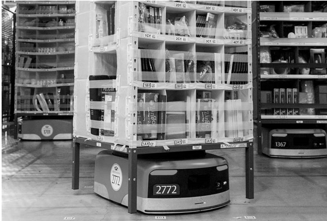
KIVA robots in an Amazon.com warehouse fulfilling a goods-to-picker strategy. Source: Amazon Robotics
