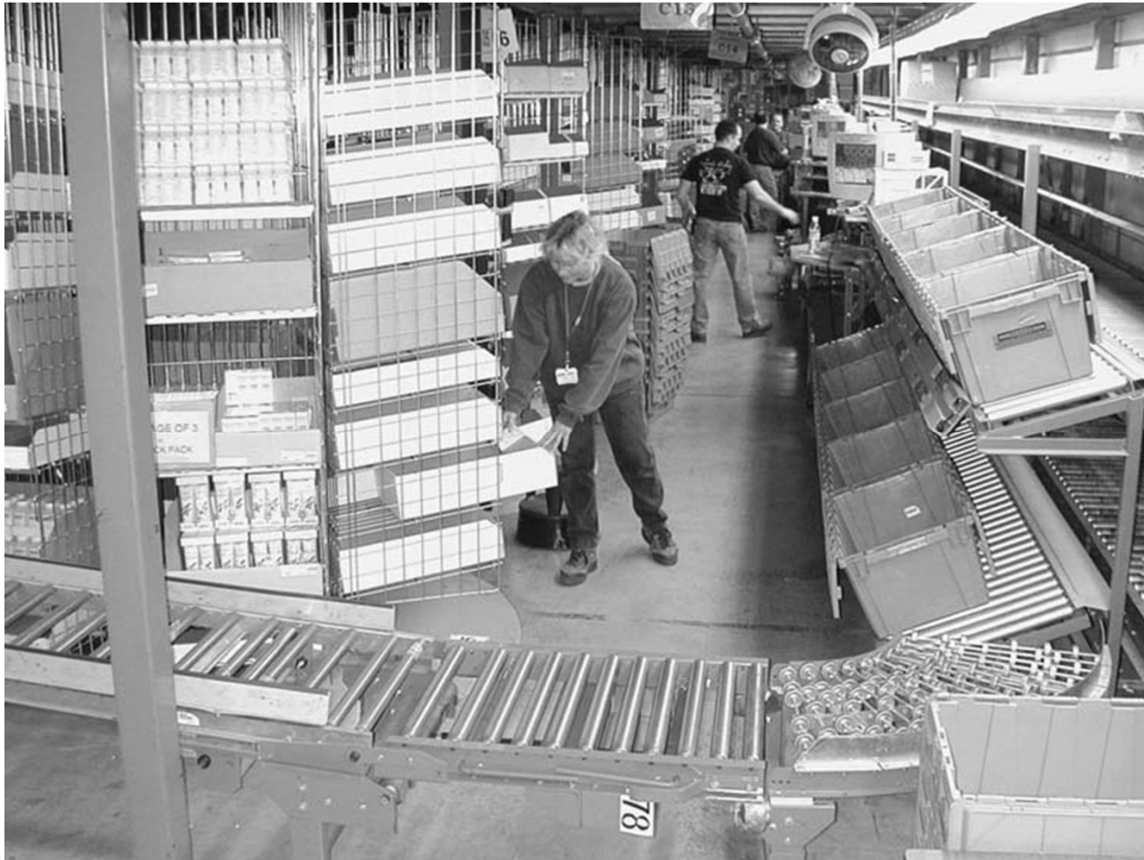
A horizontal carousel can be used in a goods-to-picker strategy. Source: unknown
