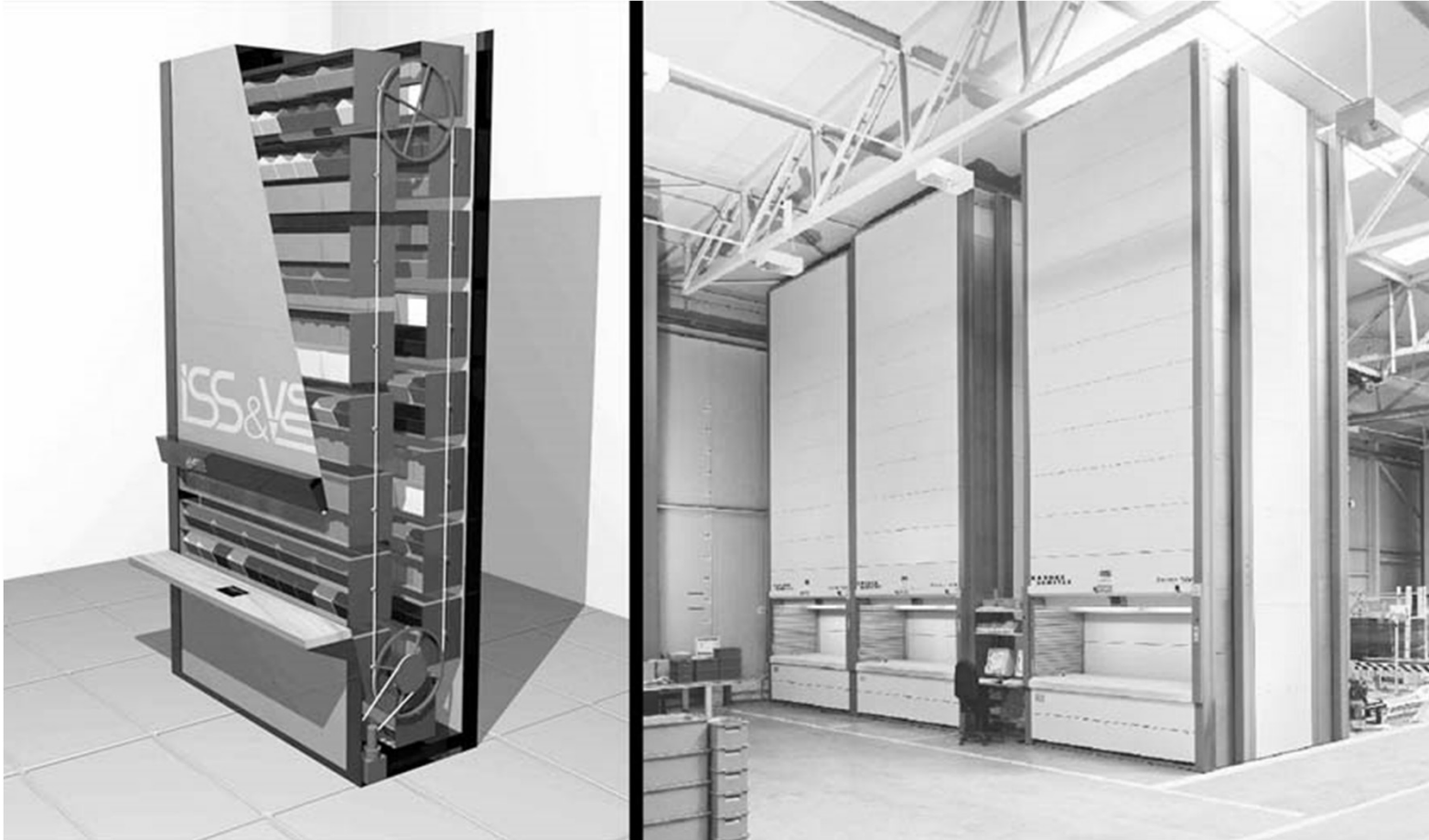
Vertical carousel system for small parts Source: Patrick VanRuymbeke
