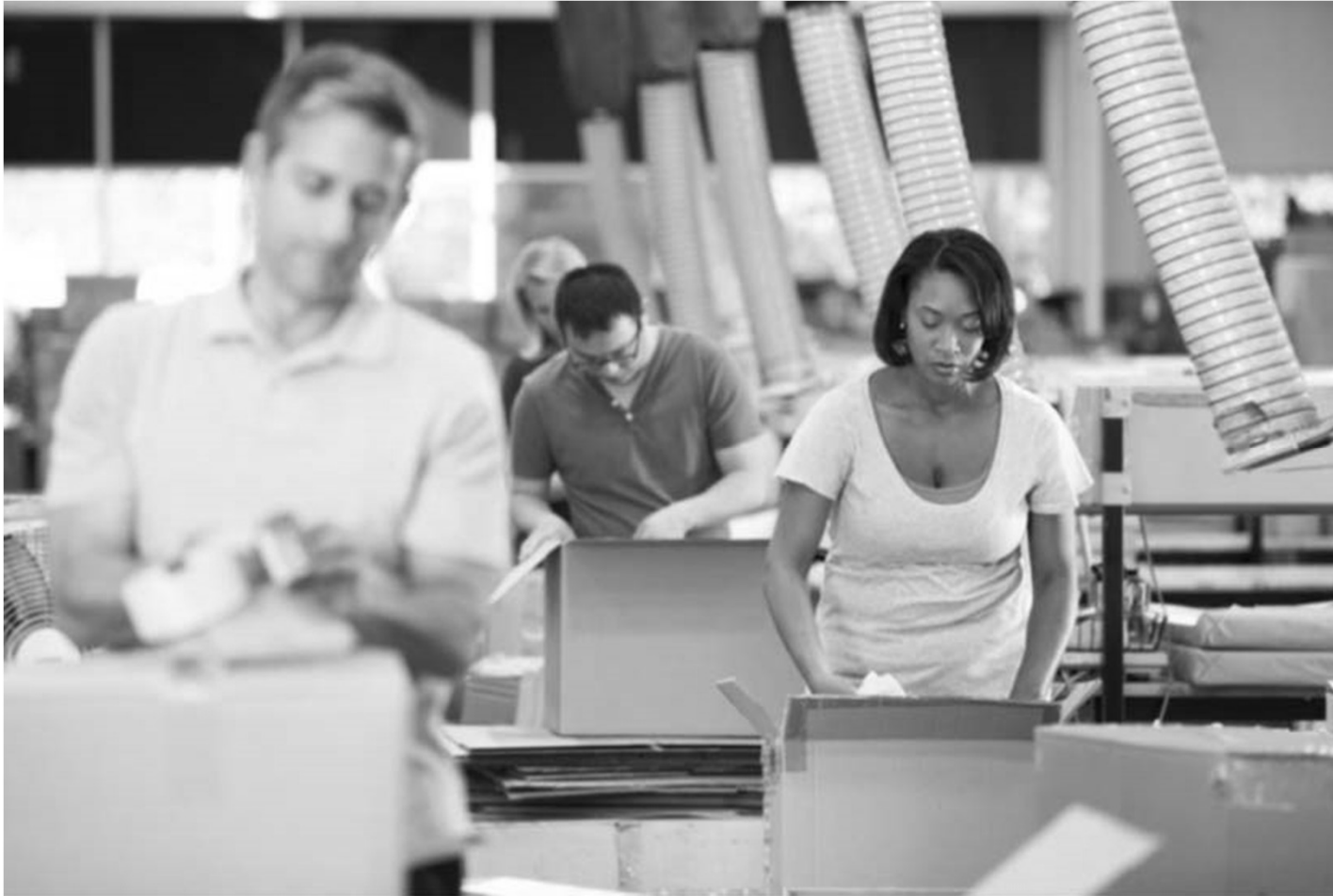
Packaging the goods that have been collected by pickers. The chutes (on the right) provide packing pellets to fill the boxes.
