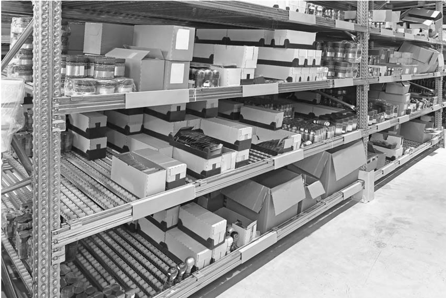
A rolling-rack system for small parts in a warehouse in the United Kingdom Source: Baloncici
