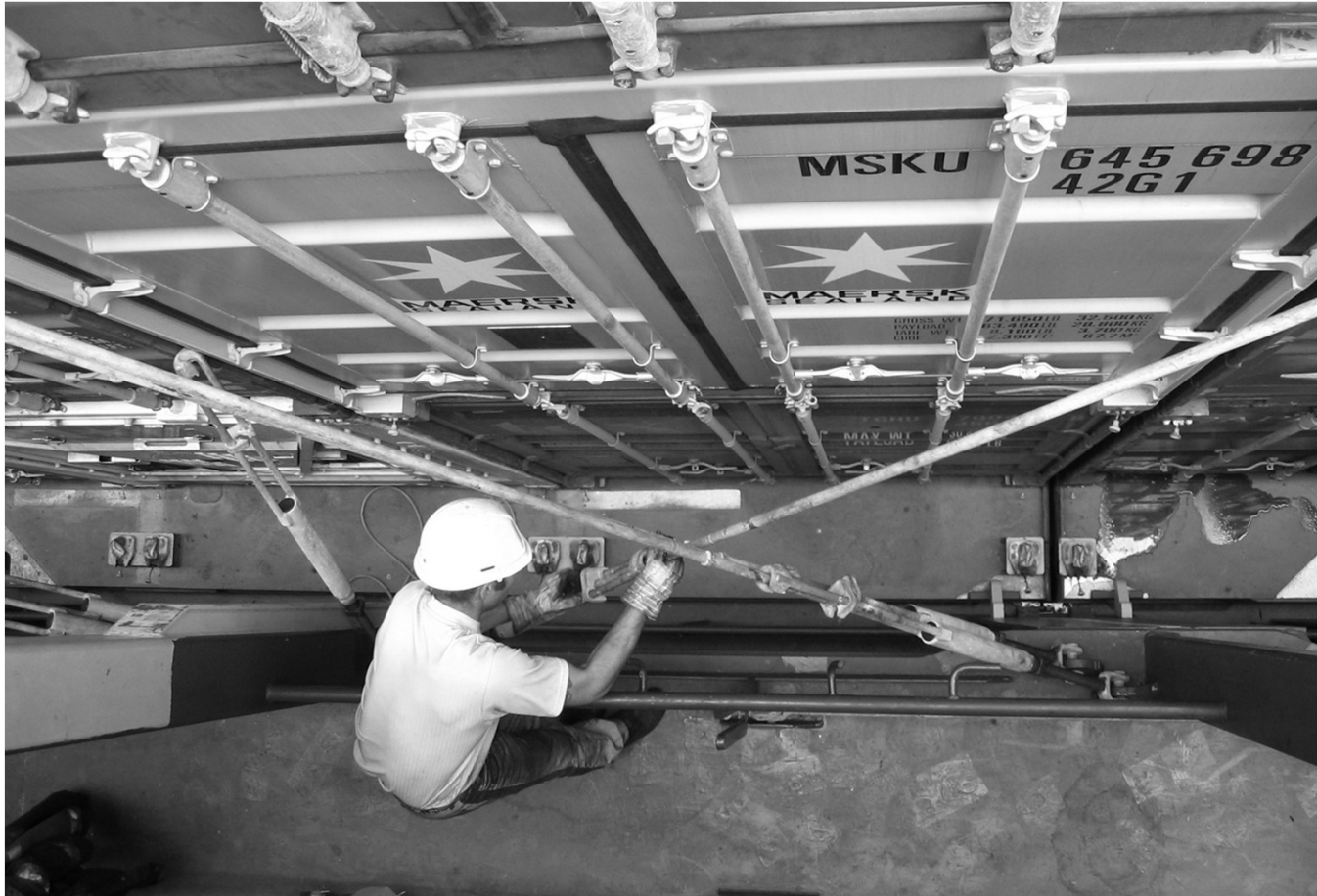
Containers at the bottom of a stack are attached to the ship by lash bars. Source: unknown
