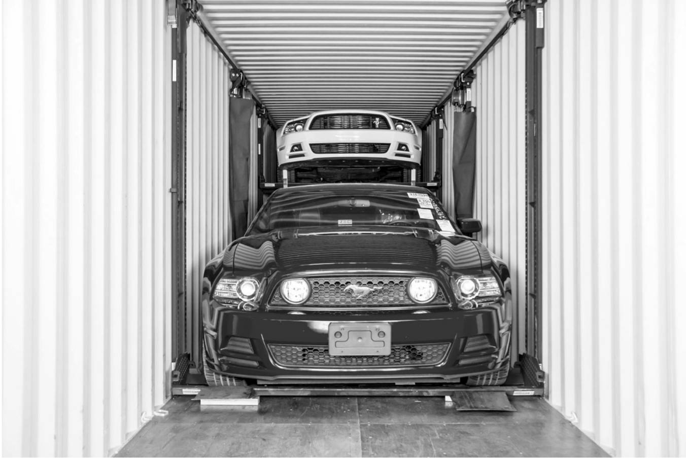
Containers can be equipped with racks for roll-on roll-off cargo. Source: CFR Rinkens
