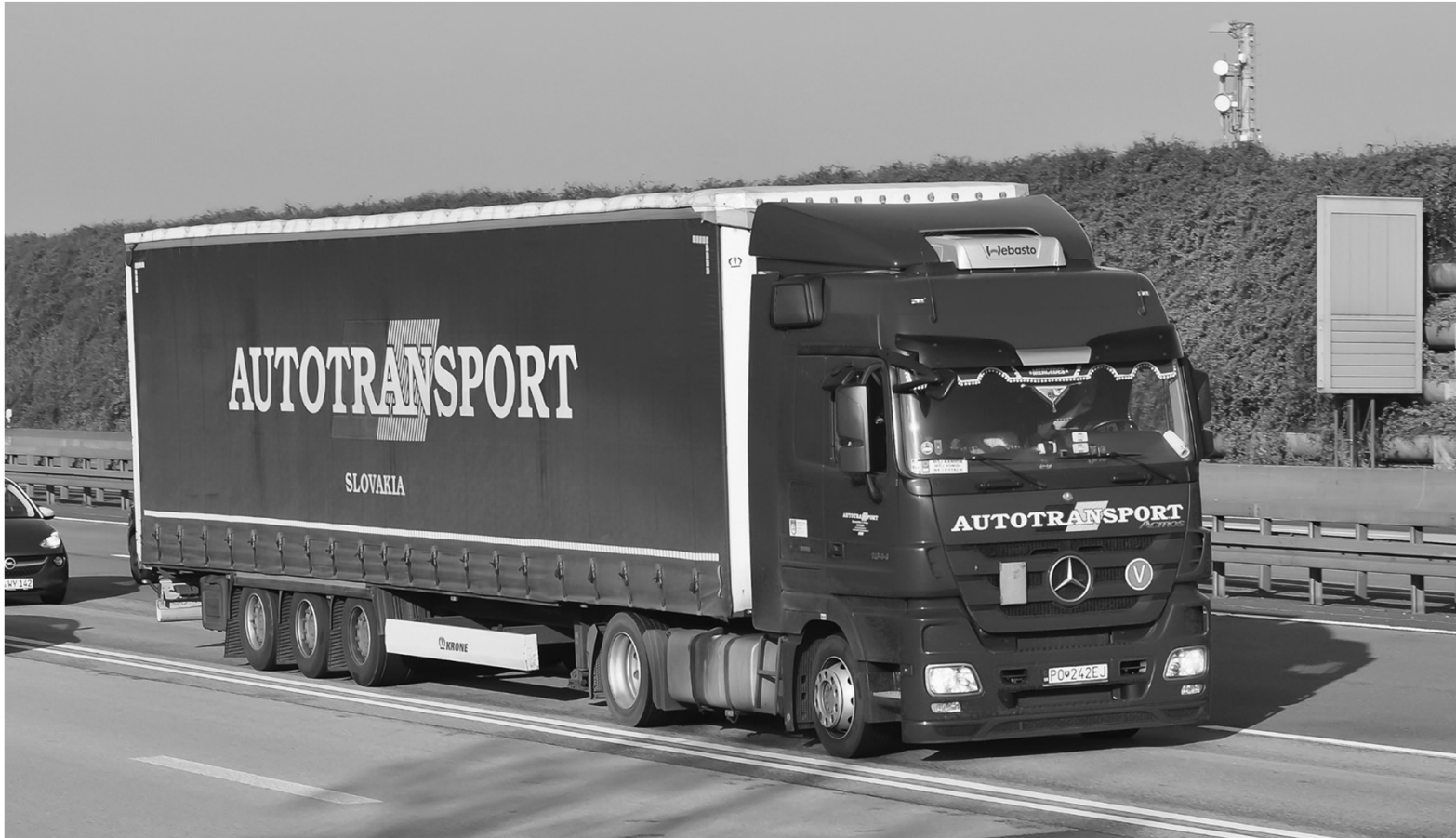
A European truck is limited in its overall length. The tractor is therefore as small as possible. Source: Vytautas Kielaitis
