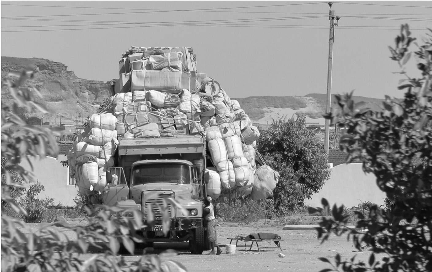
In some developing countries, the weight capacity of trucks is routinely exceeded. Source: Lutz Heckenberger
