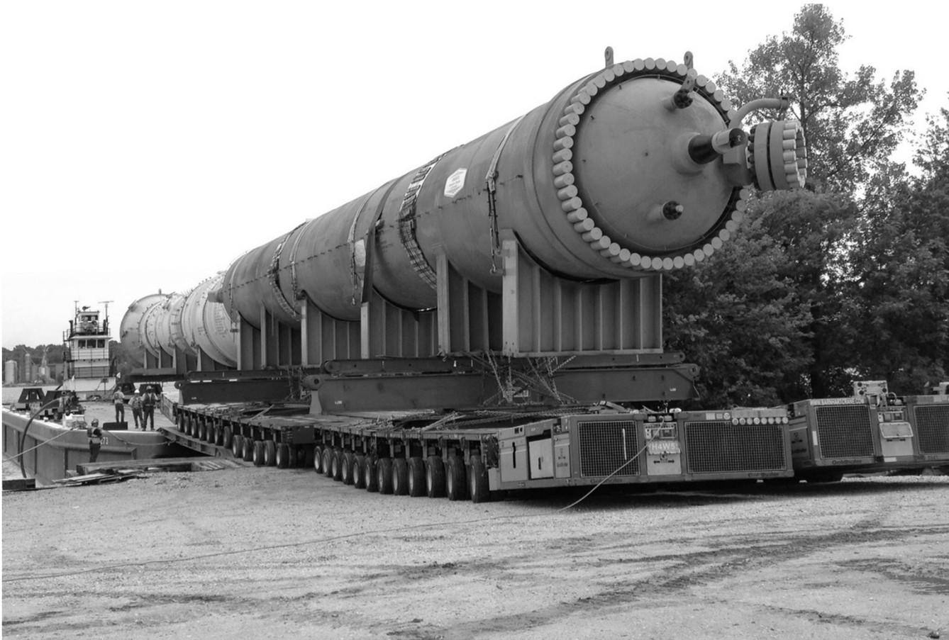
Project cargo requires careful planning because of its unusual size or weight. Source: unknown
