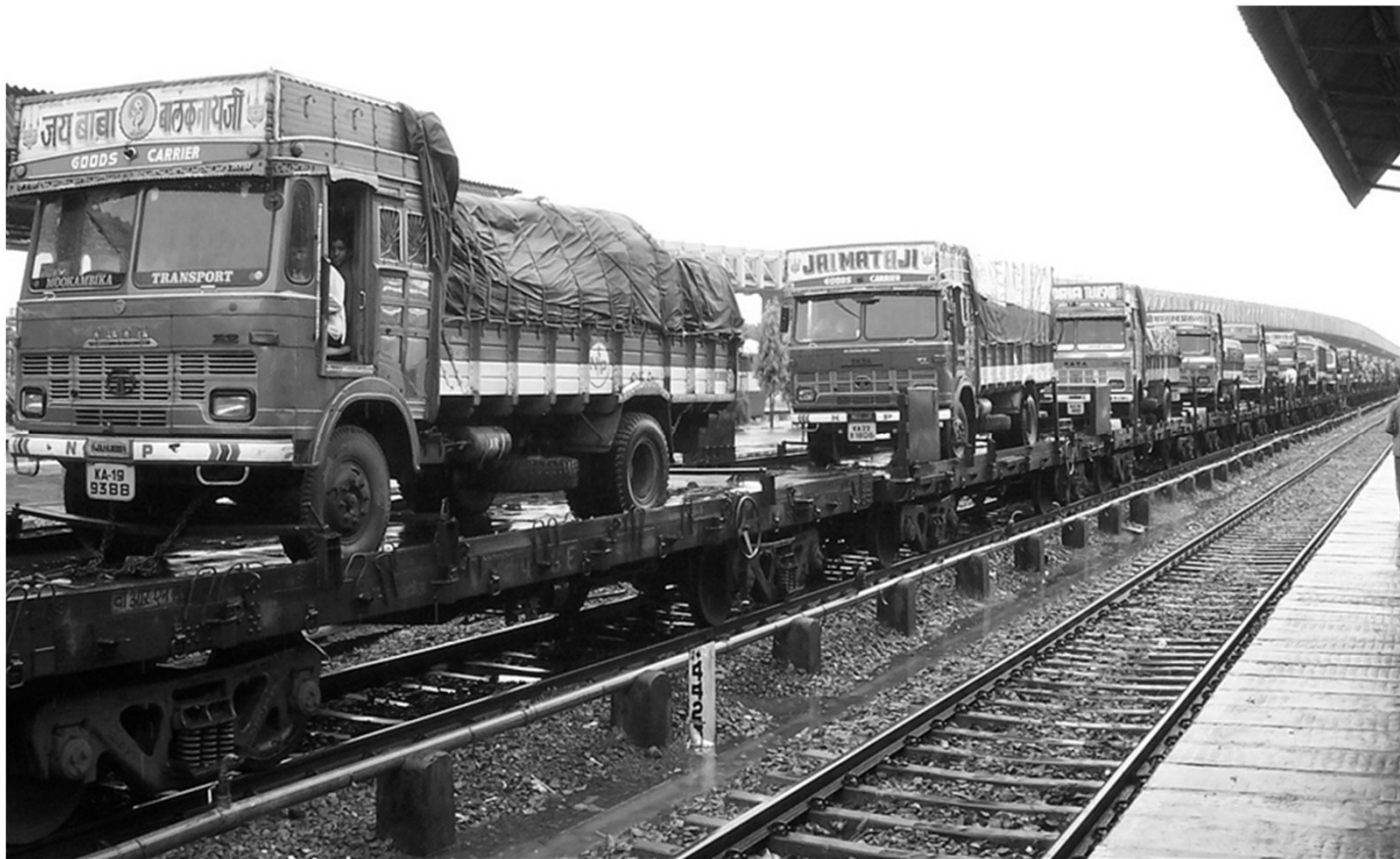
Indian trucks can also travel on railcars, to avoid congestions on intercity highways. Source: unknown
