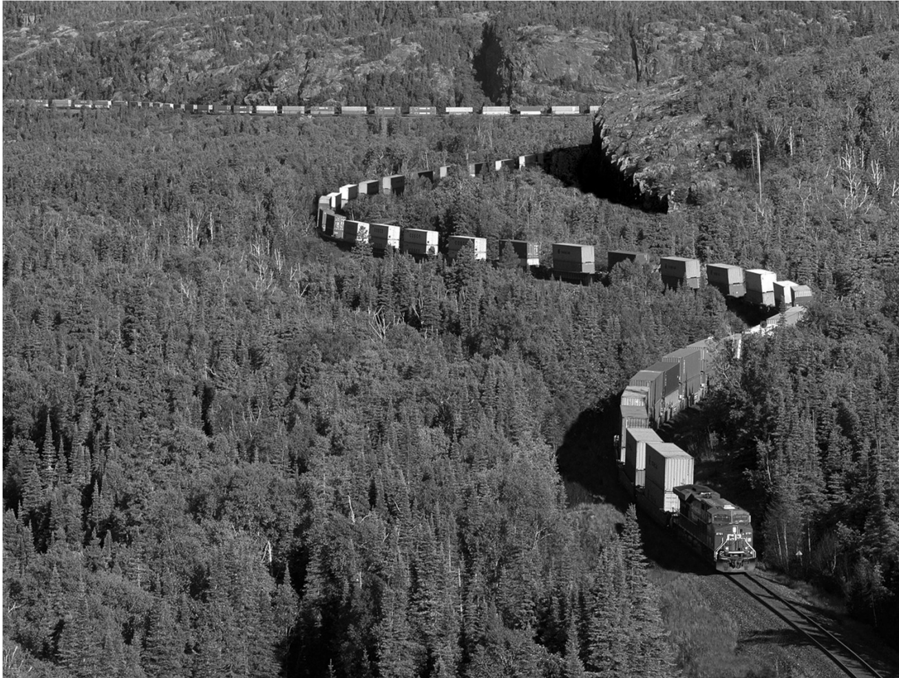
North-American railroads transport containers in double-stack railcars. Source: Canadian Pacific Railroad
