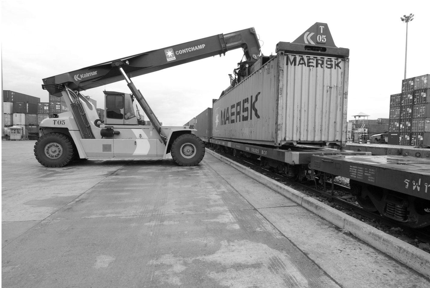
A stacker moving a container onto a train in an intermodal terminal.
