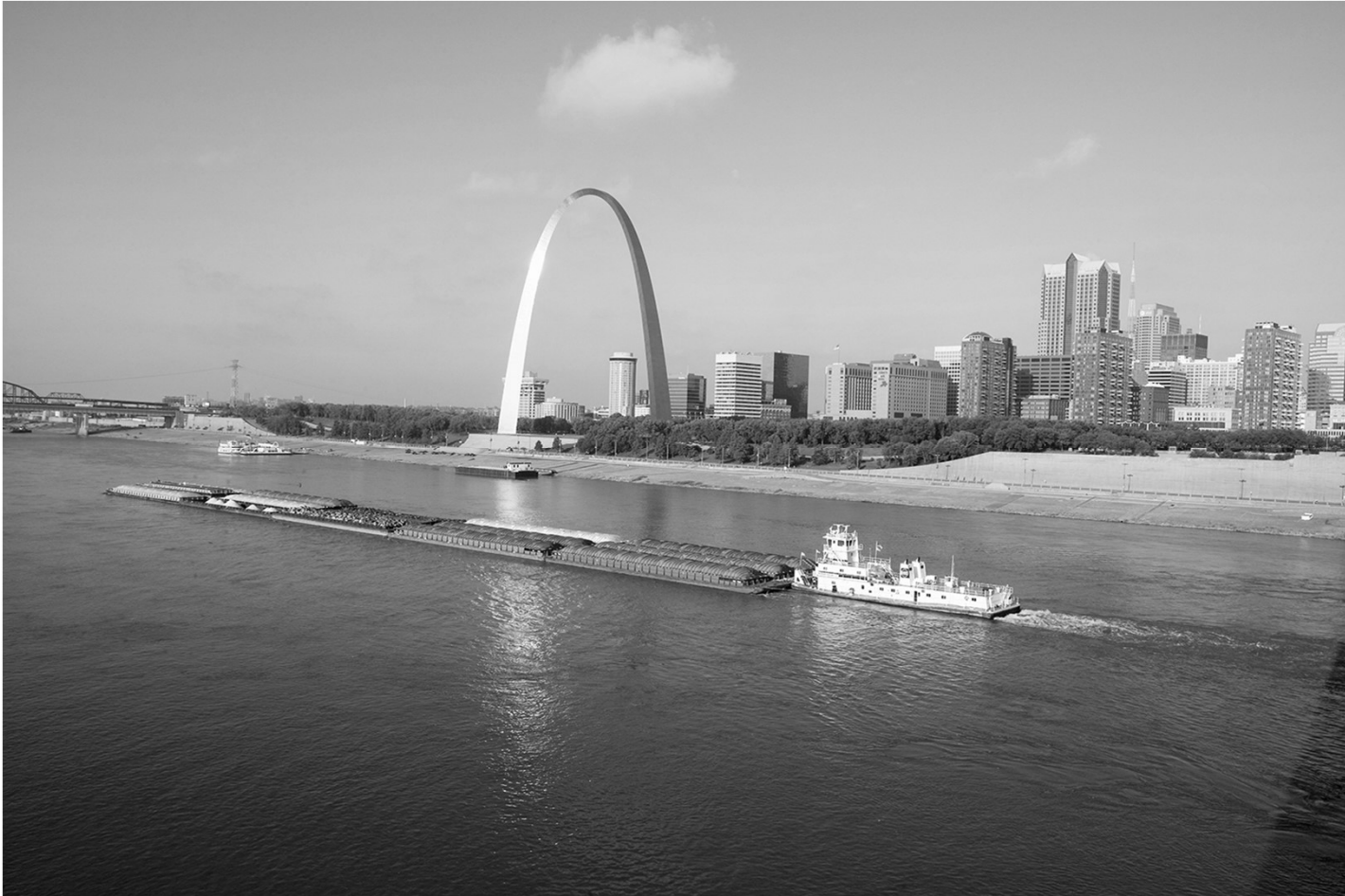
Barges on the Mississippi River. In the United States, they are not self propelled. Source: Joseph Sohm
