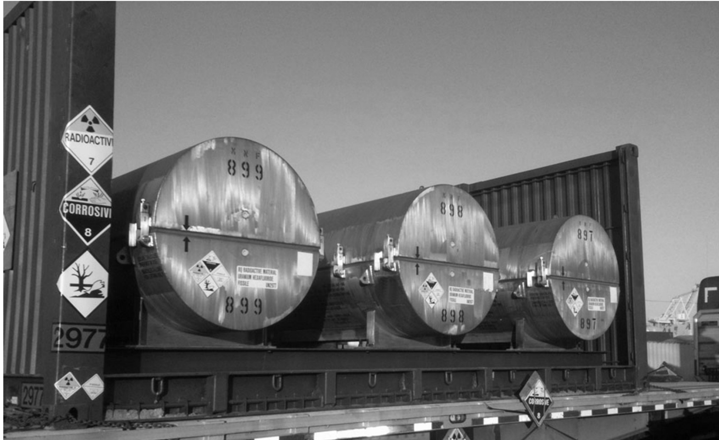
A shipment of uranium hexafluoride, a radioactive acid that is dangerous to the environment, duly labeled for international transport by ocean.
