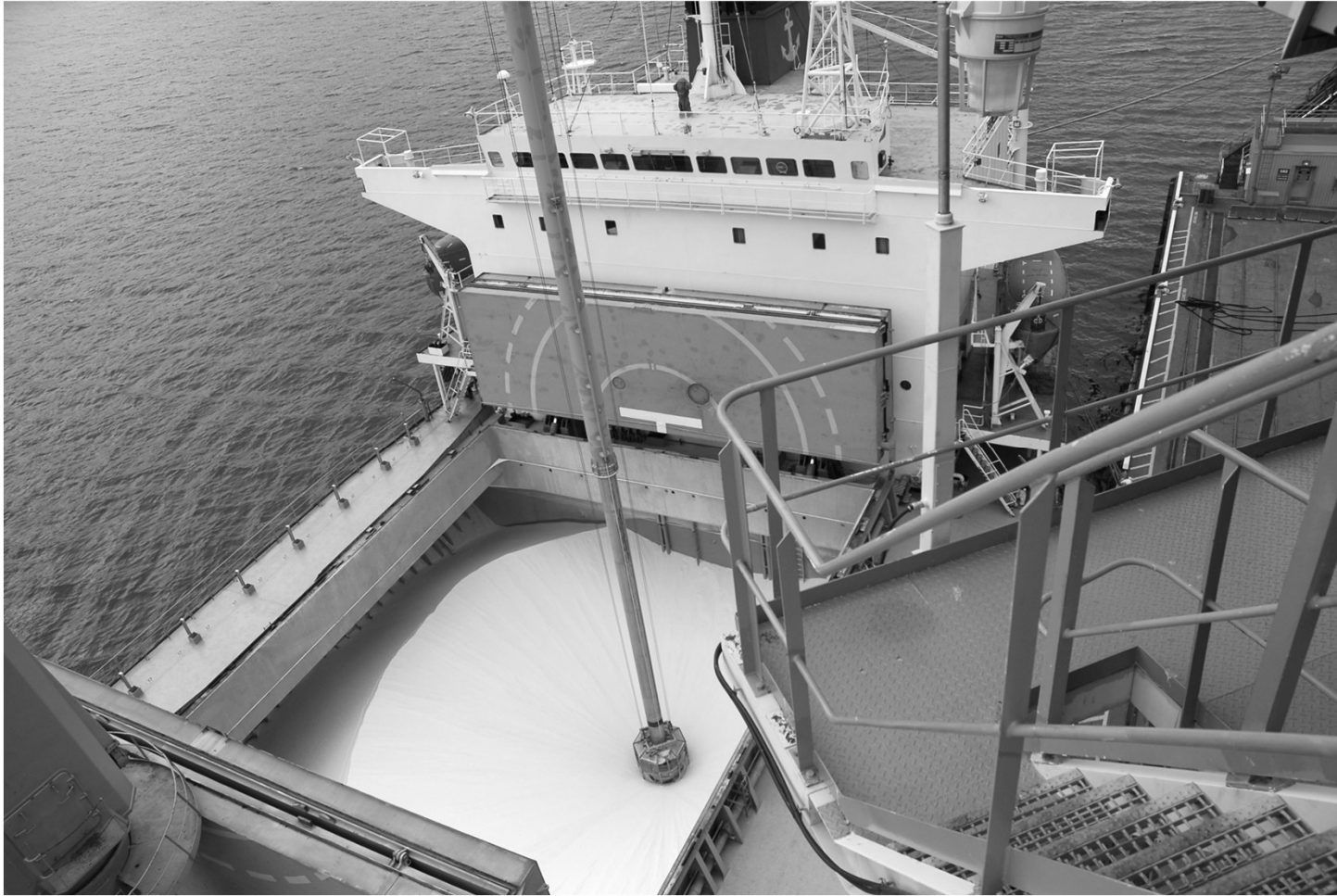
Alumina being unloaded using a vacuum pump.
