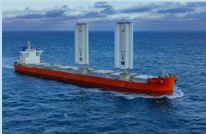
BAR TECHNOLOGIES: Although it did not secure funding from Britain, it received $1.5m from the European Horizon programme to install a rigid wing system on the Cargill-chartered 81,000-dwt bulker Pyxis Ocean (built 2017) Photo: Cargill
